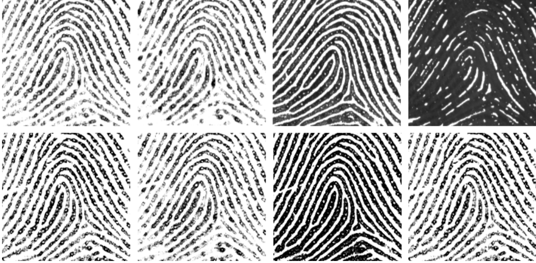
Figure 9.3: Collected fingerprint sample excerpts. treatment from left to right: normal, dry, cream and water; top row shows samples acquired using a sensor from \mathcal{G}_1 , bottom – \mathcal{G}_2 . Measured moisture from left to right: 630, 610, 778 and 999.
