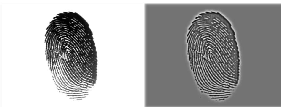
Figure 7.8: Example of normalization process using image from FVC 2004 [168]. (a) is the input image and (b) is the enhanced version.
