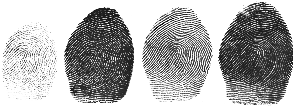
Figure 9.1: Fingerprint samples acquired from same finger with skin subjectively perceived as (left to right): dry (62.5%), wet (99.9%), normally moist (84.6%) and normally moist (84.6%) with finger strongly pressed on the sensor.
