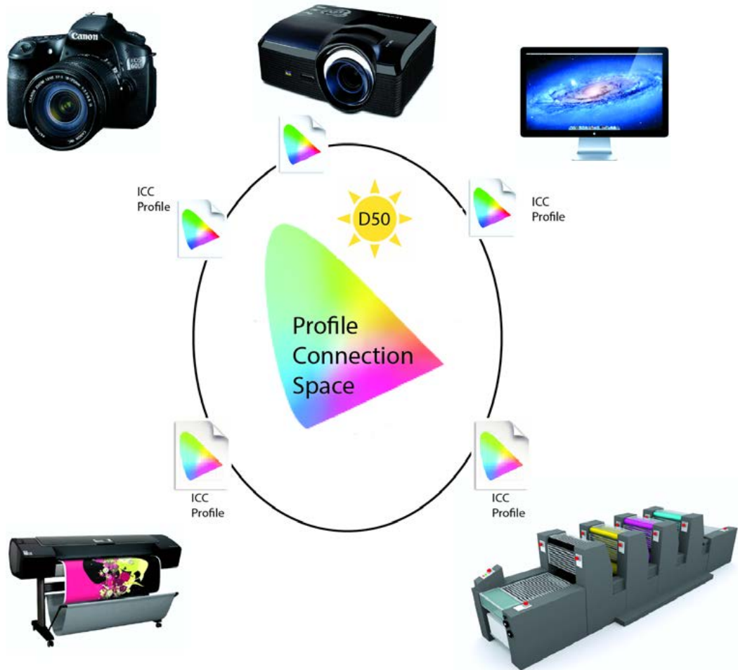
Figure 1.* Commonly used colorimetric reproduction workflow (ICC). Devices communicate via common colour space (PCS), usually CIE L^*a^*b^* space, under the fixed illumination conditions and the standard observer (CIE Standard 1931 Colorimetric Observer).
