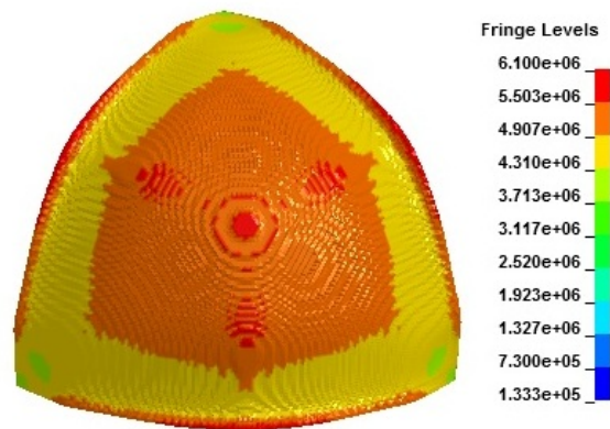
Figure 8.17: Pressure variations at the expansion wave, 1/8 symmetry model at t=4.98E-5s , Element length=1.98mm
