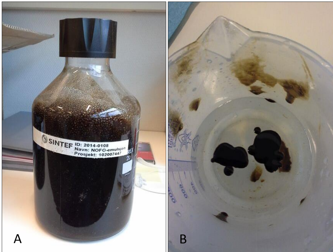
Figure 20: Crude-oil emulsion (A) crude oil emulsion sample, (B) drop of crude oil emulsion into water to check the type of emulsion.
