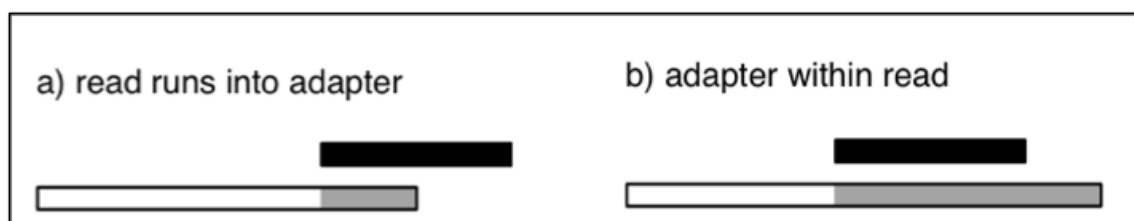
Figure 2.11: Adapter alignment scenarios. White rectangles are reads, black are adapters and grey are segments removed. Image adapted and modified from Martin (2011).
