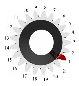
Figure 19. Front view of the sun gear in the SIMPACK model.
