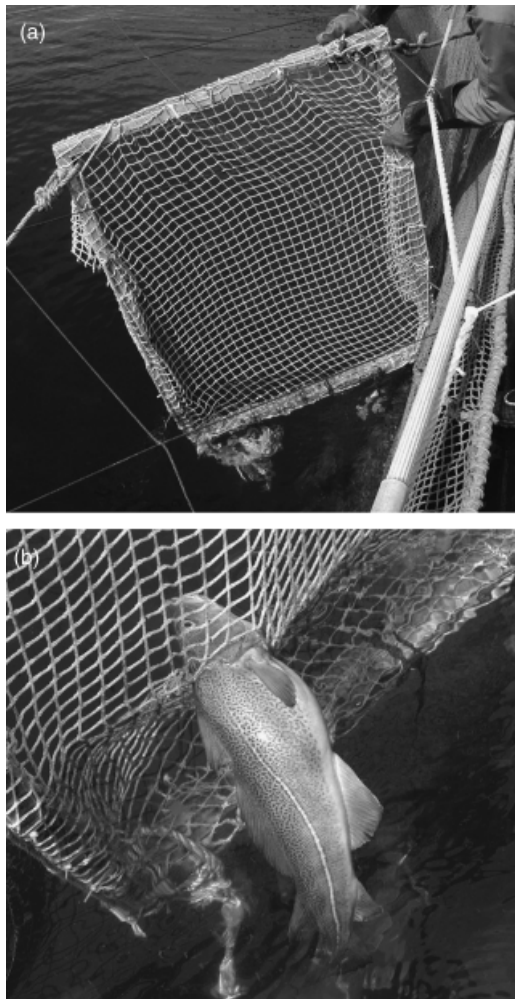
Figure 2 (a) Launch of a test net panel in a commercial cod sea cage and (b) an escape attempt through a pre-damaged hole (one-twine cut) in a test net panel by a 1 kg fish. The panel had been in the cage for 1 month.
