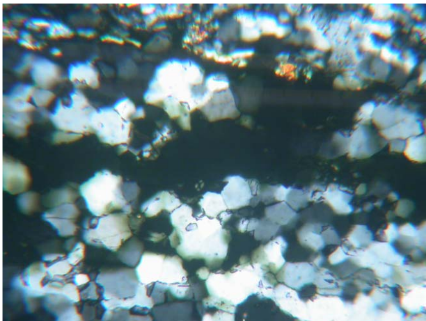
Photo 4 CAN 1 thin section. Same as photo 3. Polarized light. Dissolution of quartz crystals in reacted aggregate. Length of photo is 0.5 mm
