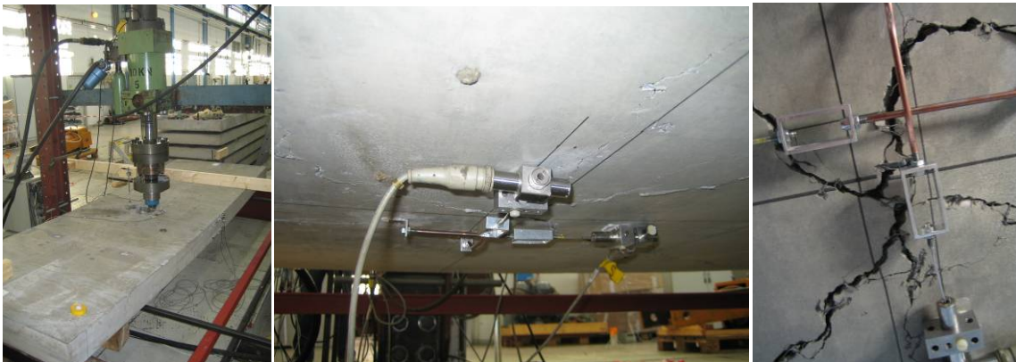
Figure 9.5: a) Loading. b) Cracks initiated under the load. c) Cracks under the load after failure.
