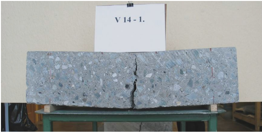
Figure 5.8: One crack developed in the midsection for all beams, here beam W14-1.
