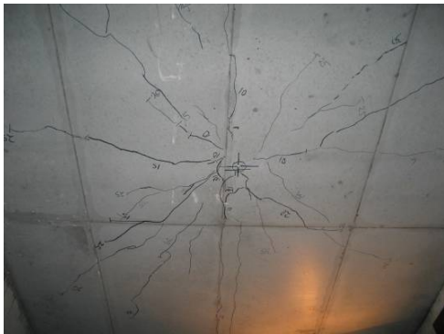
Figure 10.17: Left: Slab II after loading, seen from below. The cracks were marked by a tracer at each load step. Right: Crack below Slab III, illustrating fibre bridging. Small pieces of concrete were spalling off around the fibres near the surface.
