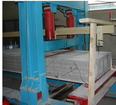
Figure 10.2: Dimensions and loading of the hollow core elements. The number of prestressing steel was 10.
