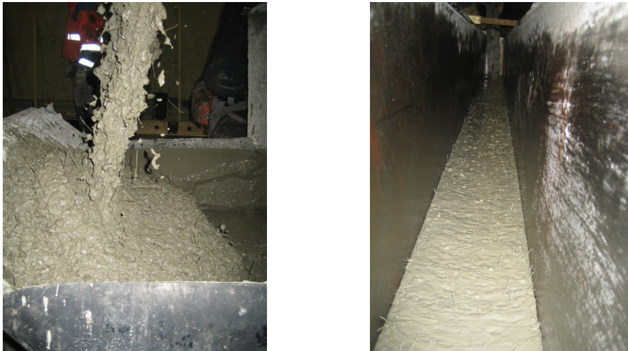
Figure 10.20: Left: The fibre concrete was poured in a pump. Right: Wall4 with synthetic fibres from the opposite side of the casting point. The picture shows that tendencies of pasta separation occurred.
