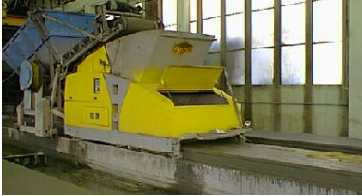
Figure 10.1: Casting of hollow core sections. The concrete is filled and compressed through the machine. The cores are made by rotating cylinders. [Contiga 2007]
