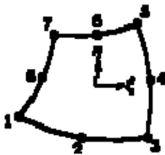
Figure 6.23: Plane stress element CQ16M in DIANA [De Witte et al. 2002]
