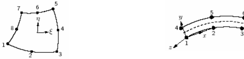
Figure 8.12: a) CQ16M eight-node element, b) CL12I interface element. The opposite nodes may overlap: 1 and 4, 2 and 5, 3 and 6.
