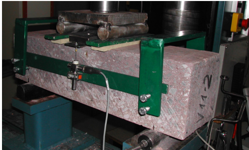
Figure 10.9: 4point bending of beams (150 x 150 x 600mm).
