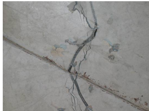
Figure 10.17: Left: Slab II after loading, seen from below. The cracks were marked by a tracer at each load step. Right: Crack below Slab III, illustrating fibre bridging. Small pieces of concrete were spalling off around the fibres near the surface.
