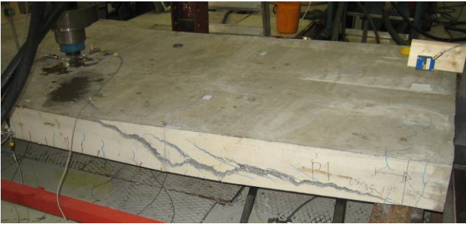
Figure 9.6: Slab S1B. Anchorage/shear failure.
