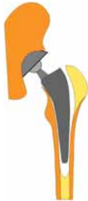
Figure 2: A femoral component inserted in the femoral canal. The acetabular cup is fixed in the pelvic bone and receives the artificial femoral head.
