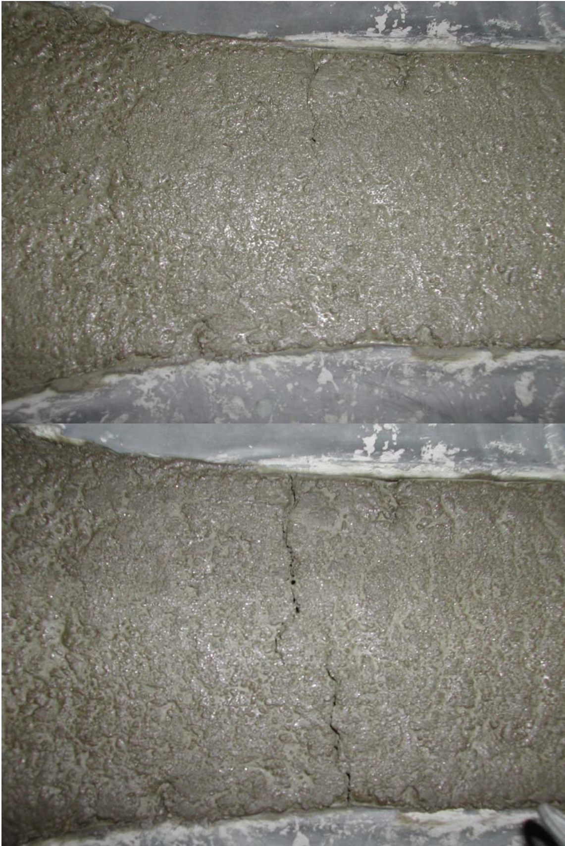
Fig 8.4 Crack propagation of a restrained specimens (100 mm in width) exposed to 50 % RH and 21 °C and 5 m/s wind velocity. Upper picture taken at 10 minutes of drying, lower at 90 minutes.
