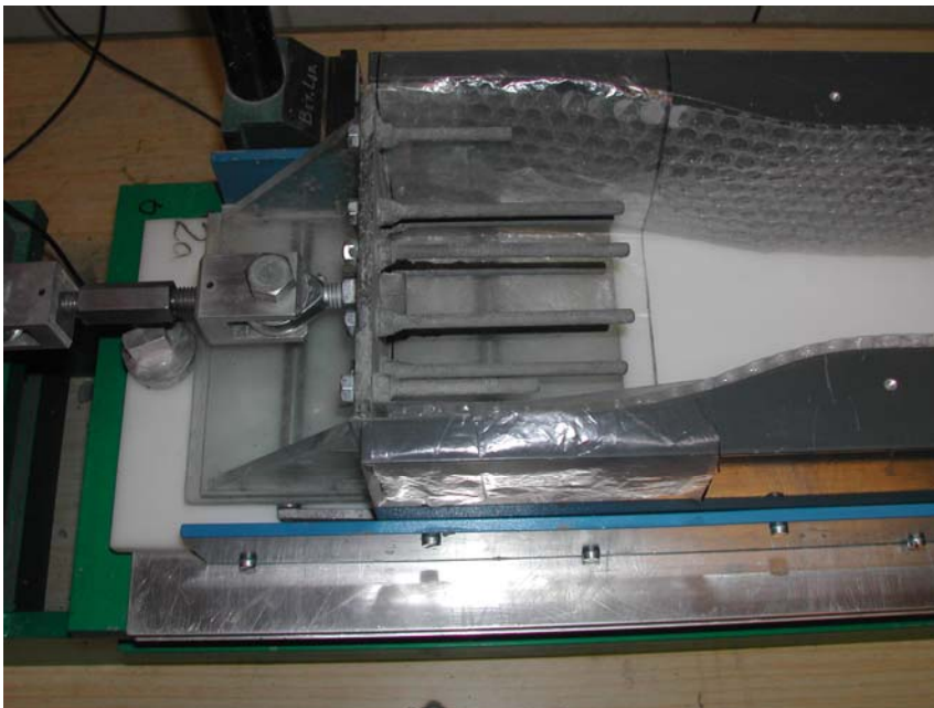
Fig. 7.4 Picture of end section with rollers.
