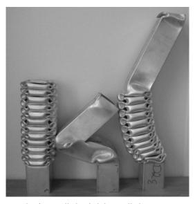
Figure 1-2 Collapse modes for axially loaded thin-walled components; progressive, global and transition mode.
