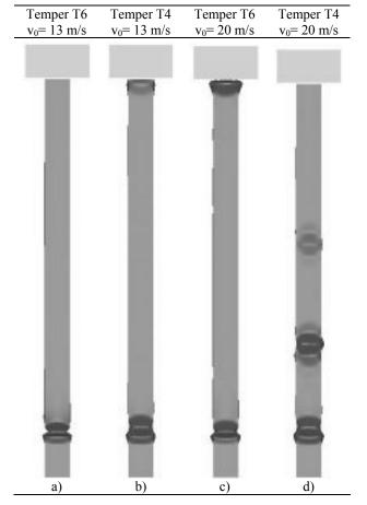
Behaviour of aluminium extrusions subjected to axial loading
