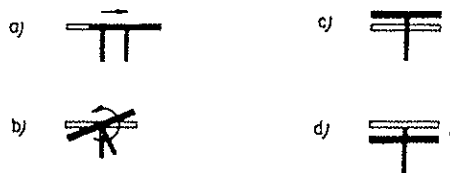
Fig. 3.8.2 Possible buckling modes for the tee section in compression. [Figure from Höglund (1970)]
