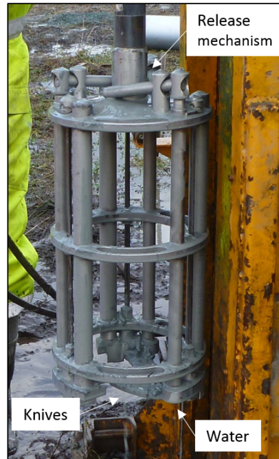
Figure 4.1: The different elements indicated on the mini block sampler [9]
