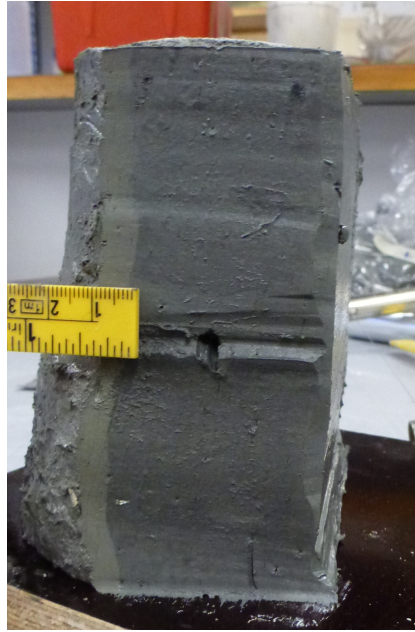
Figure 7.2: Discoloration in the mini block sample periphery (Photo: Rikke N Bryntesen)
