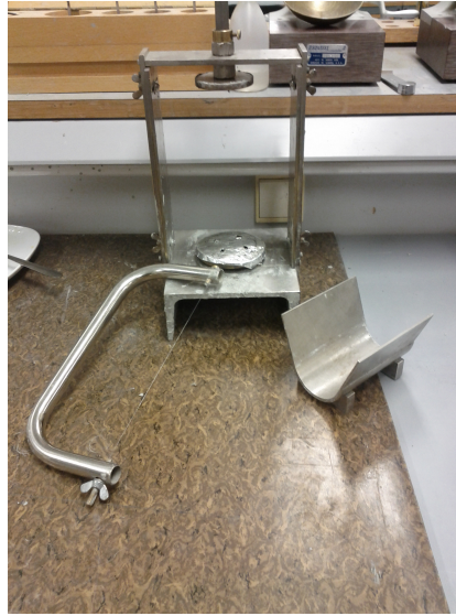
Figure 6.8: Equipment for triaxial specimen preparation. (Photo: Rikke N. Bryntesen)
