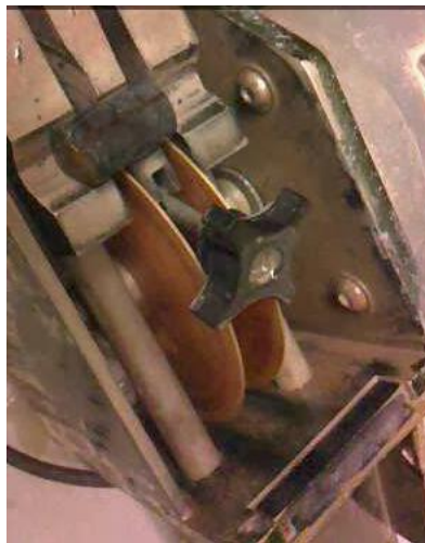
Figure 7.1-2: cutting of cores with brass blades.
