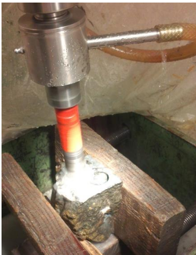
Figure 7.1-1: core drilling of samples.
