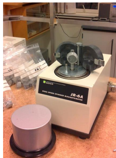
Figure 7.2-3: NRM JR-6 spinner magnetometer.
