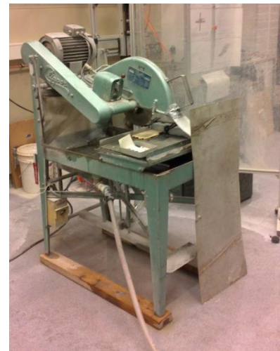
Figure 7.1-3: cutting and re-cutting of cores into specimens.
