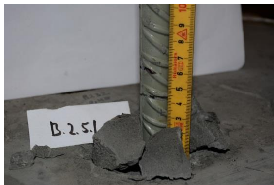
Figure 41 – The black mark on the bolt is to measure the pull-out length. The length is 6 cm. The bolt slid from the grout with maximum load around 120 kN.
