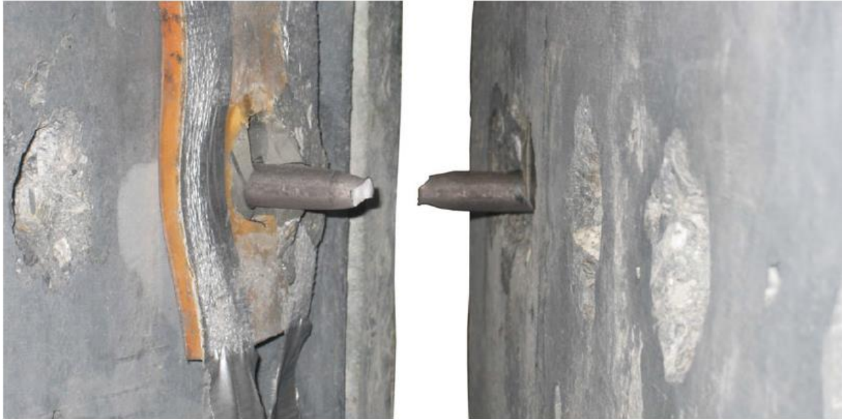
Figure 30 – Bolt OP1 after the pull-out test. The bolt failed at the displacement of 110 mm. It started to yield at 170 kN and had a tensile strength up to approximately 210 kN (Charlie and Doucet, 2011).
