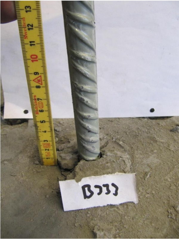
Figure 55 – The bolt was barely pulled from the grout, but was at the verge of breakage.
