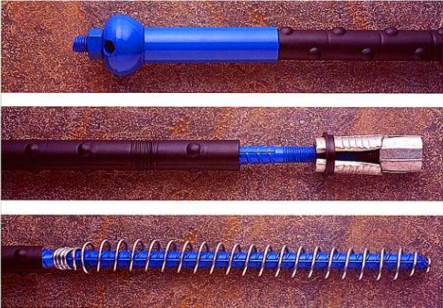
Figure 17 – CT bolt. It is a steel rebar bolt with an ordinary expansion shell and an arrangement for the injection of cement (NFF, n.d.b).
