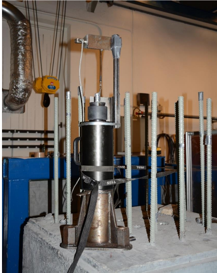
Figure 34 - The length of the bolts from the top of the concrete block up to the end of the bolts is the same for every bolt or 75 cm. The stretch length of the bolt (the length of the base and the cylinder) is however, 60 cm.
