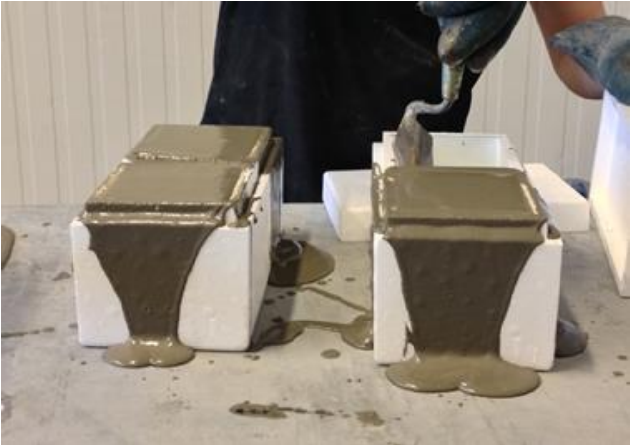
Figure 38 – 10x10 cm cubic boxes filled up with cement mortar and seven days later tested to find the uniaxial compressive strength of the grout.
