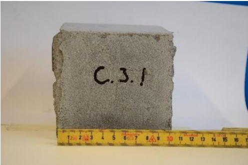
w/c ratio: 0.46 before and after
