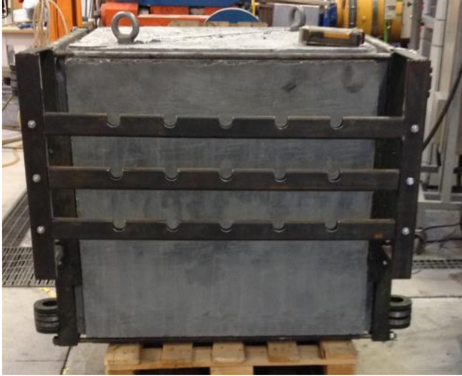
Figure 32 - Strong concrete block, USC ca. 100 MPa. The frame is put on the block and holes are drilled into the block. The diameter of the holes are 46mm and the depth varies between 40 and 50 cm.
