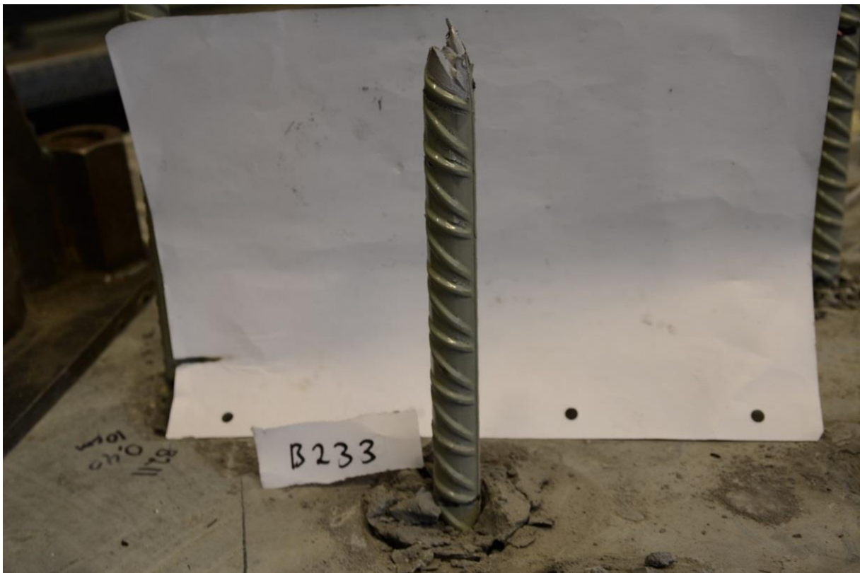
Figure 45 – The embedment length was longer than the critical length, so the bolt broke. The reduction in diameter closest to the breakage increased until the bolt broke. The maximum load reached 200 kN.
