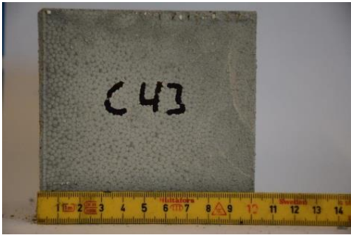
w/c ratio: 0.50 before and after
