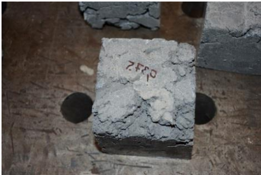
w/c ratio: 0.375. It was too dry. Not possible to make cement cubes
