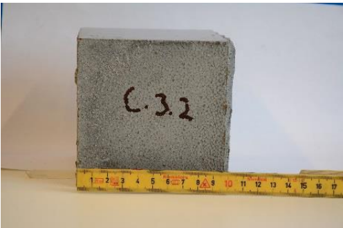
w/c ratio: 0.46 before and after
