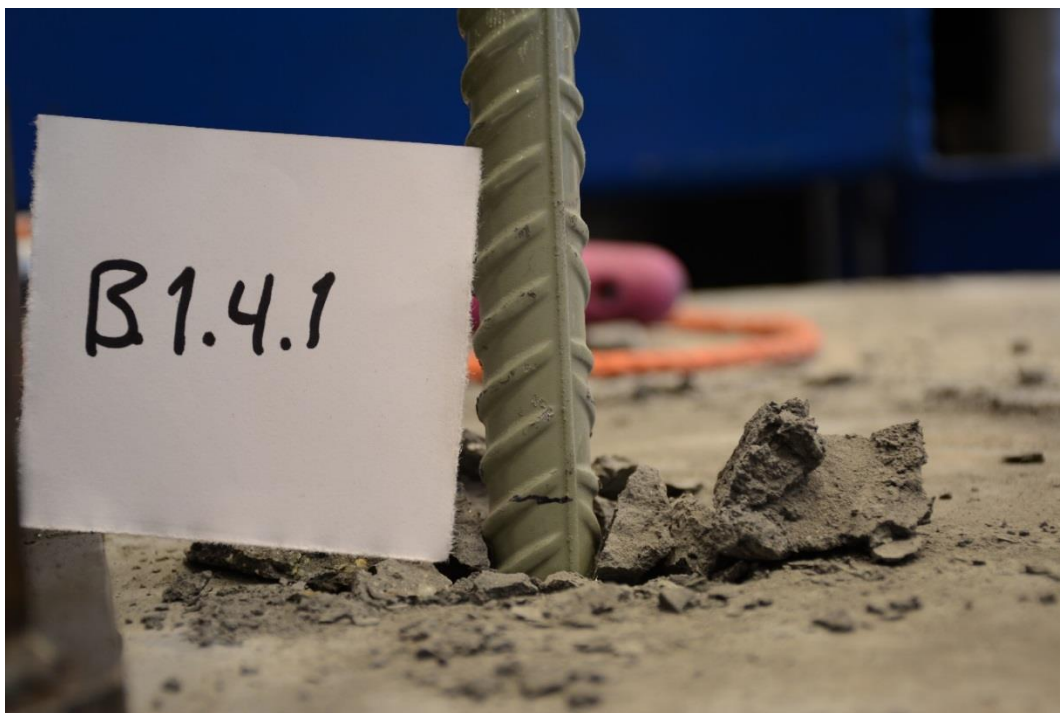
Figure 10 – Pull out test performed on rebar bolt grouted with cement mortar. The figure is taken after the testing has been performed.
