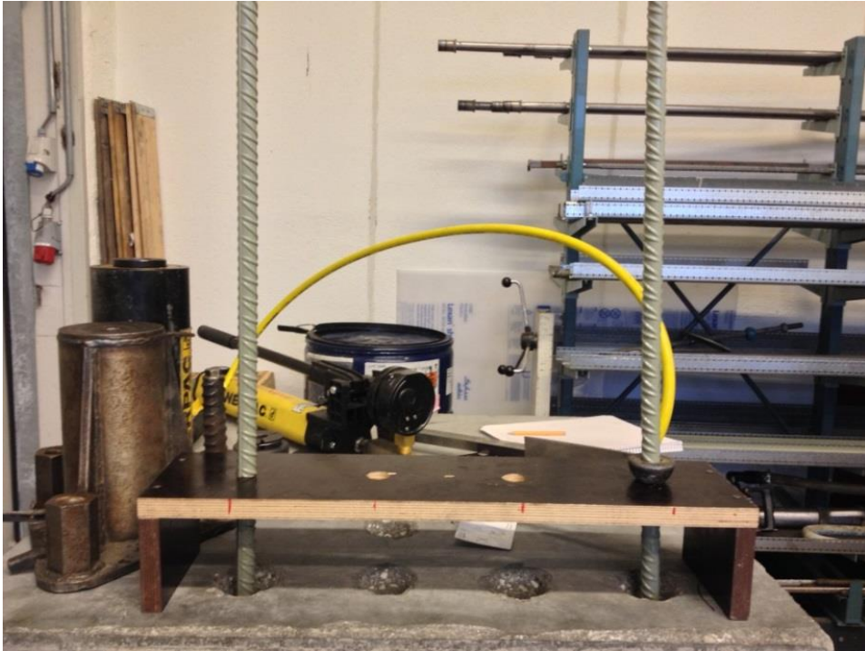
Figure 33 – Frame is used to keep the bolts from dropping into the holes and keep the vertical while the grout hardens.
