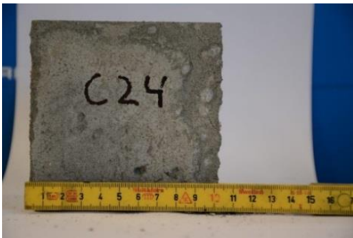
w/c ratio: 0.40 before and after
