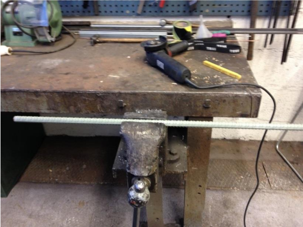
Figure 35 – The bolts were first cut and then grouted afterwards. The total length of the bolts was 75 centimeter plus the different embedment length for every bolt.
