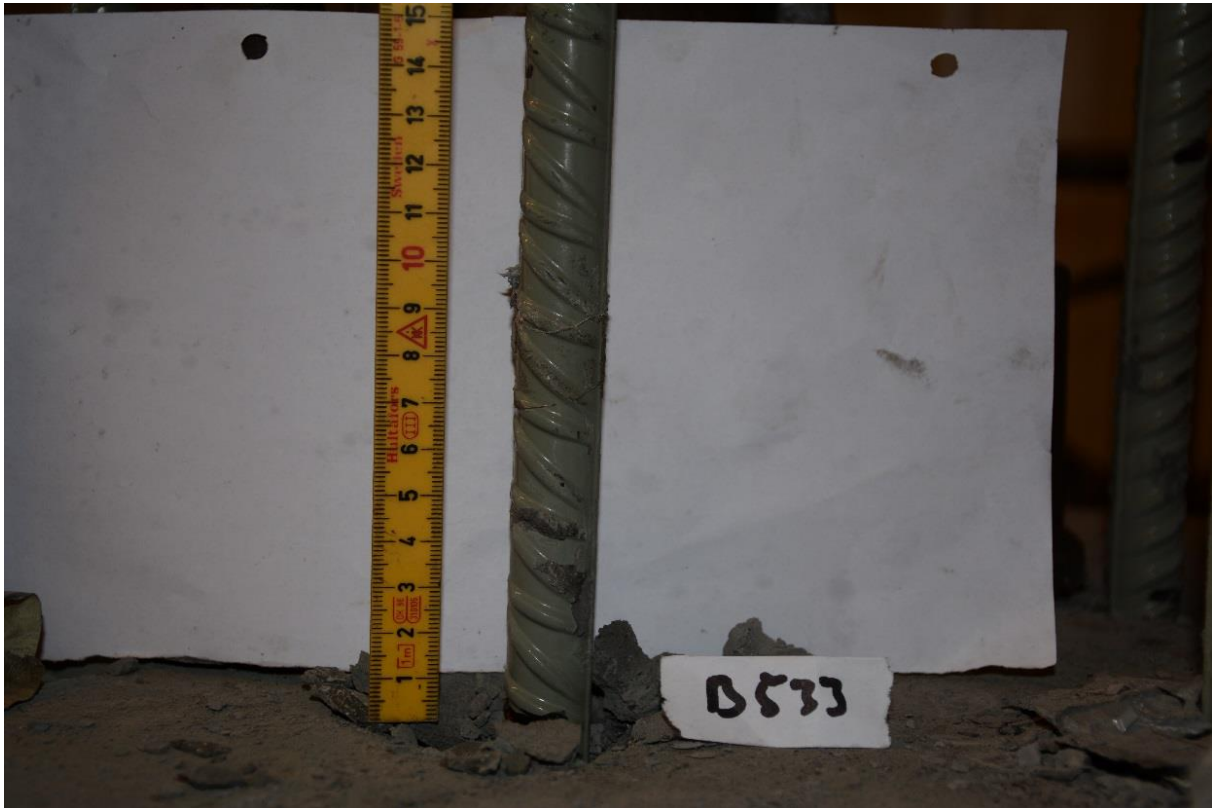
Figure 60 - the pull-out length was zero. Reduction in diameter of B533 was 0.76 mm and the stretch length elongated by 2 cm.
