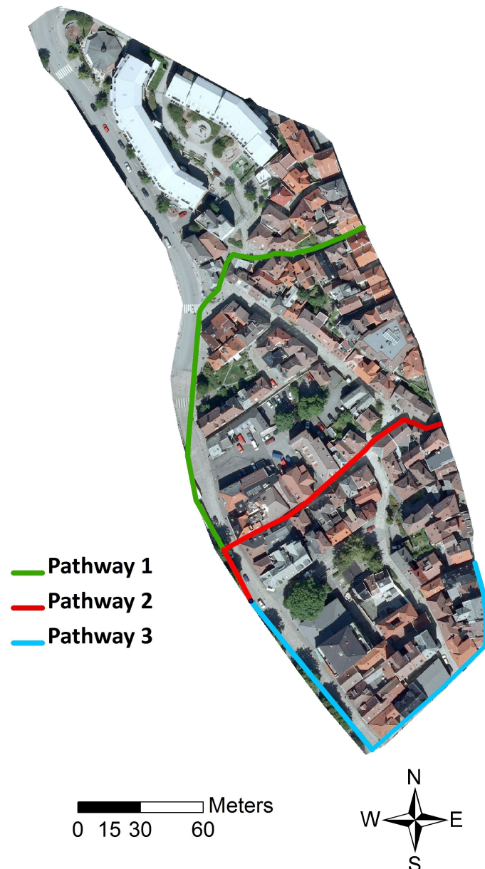
Figure 4.4: Bryggen catchment, Time of concentration calculation for three different pathways for calculation of runoff volume
