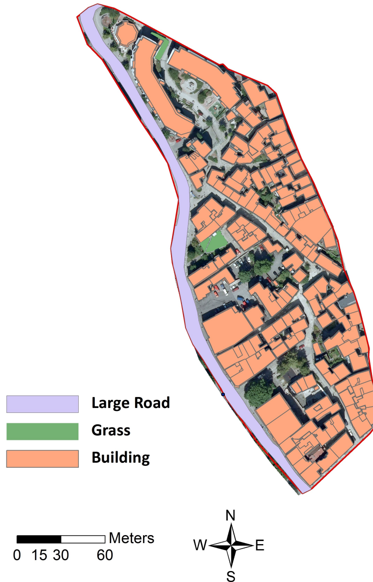
Figure 4.2: Different areas of The Bryggen catchment divided into roof, roads and grass areas.
