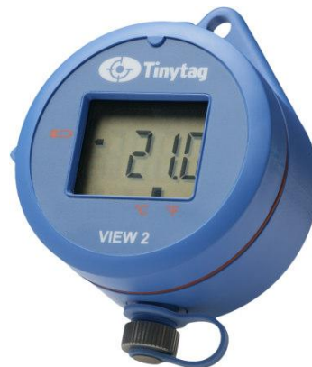
Figur 9-2 TinyTag View 2 TV-4050 (Gemini Data Loggers, 2011)
