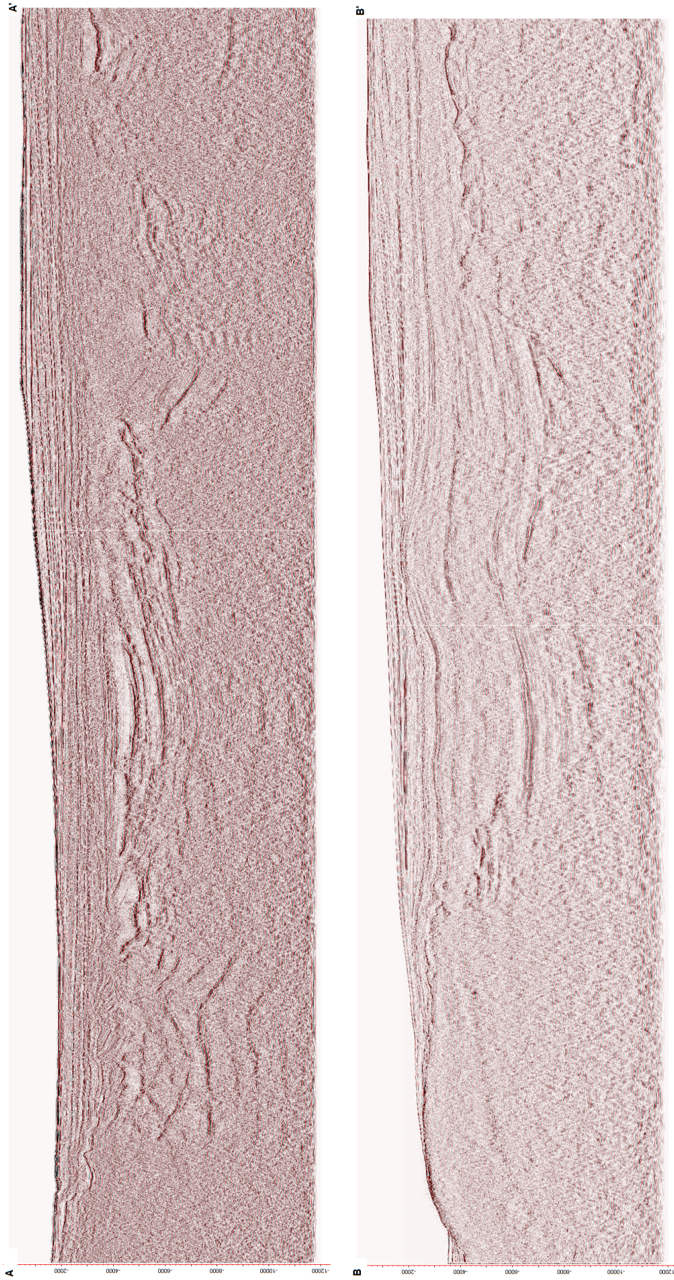
Figure 4.5: Geoseismic sections AA' and BB'. See Fig.4.1 - 4.4 for the line locations. Seismic sections are in two-way traveltime (milliseconds).
