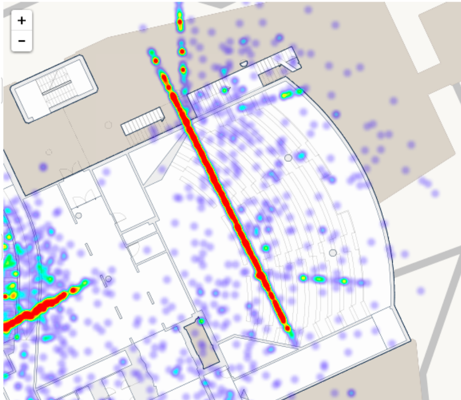
Figure 4.2: A excerpt from NTNU CMA showing the heatmap from the lecture hall R2 in Realfagbygget. Most of the positions are clustered on one line, which is probably not representing the actual movements.
