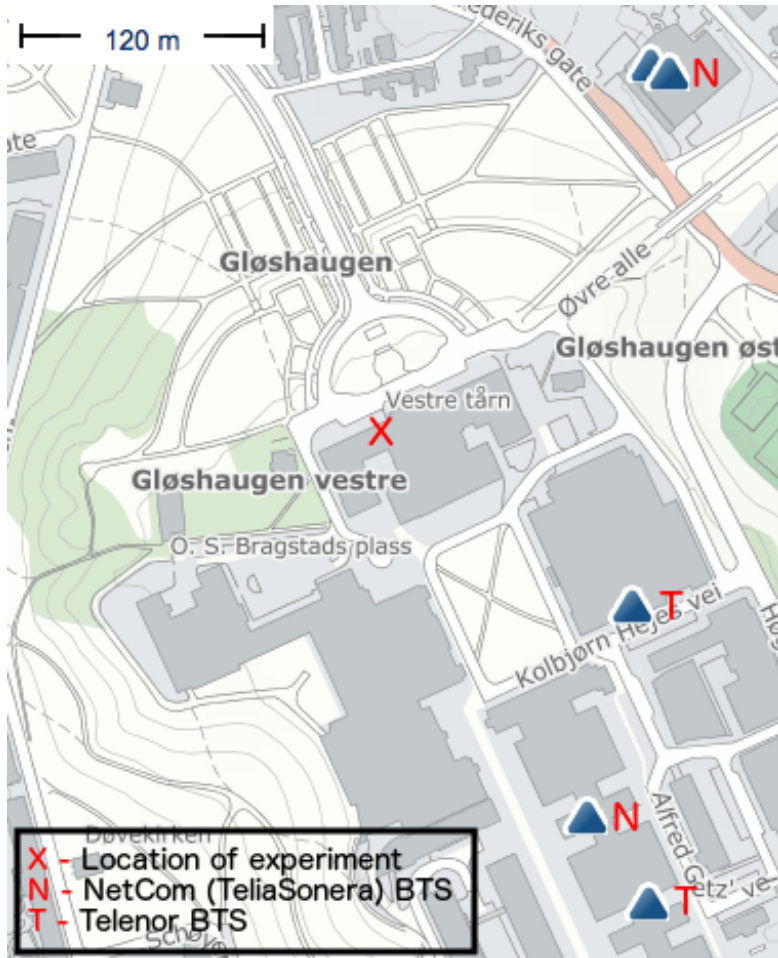
Figure 3.3: Map over the closest GSM BTSs to the location of the experiment. 'N' represents NetCom BTS, 'T' represents Telenor BTS and 'X' represents the location of where the experiment was conducted. Edited map from http://www.finnsenderen.no/ [44].
