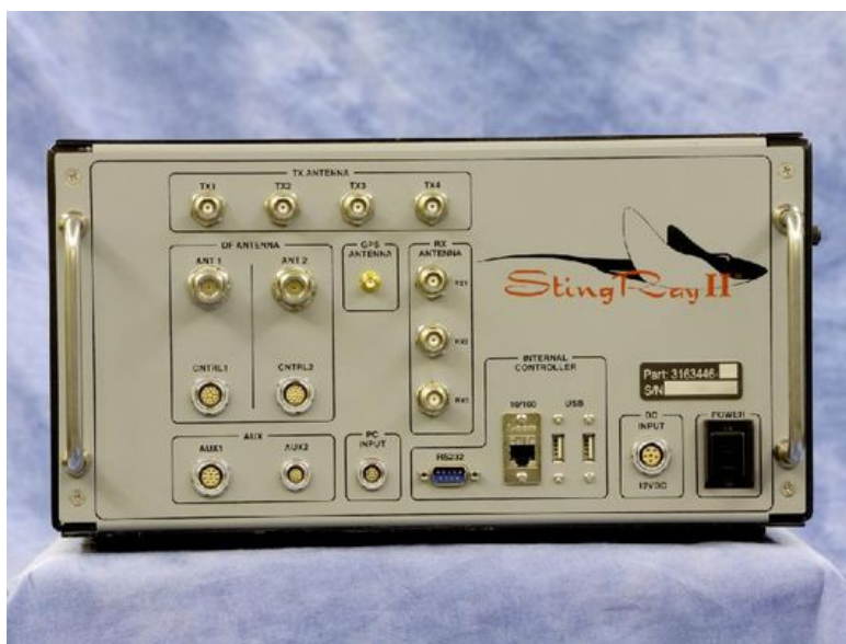
Figure 2.8: The IMSI-catcher Stingray II, produced by Harris Corp. The image is from [31].
