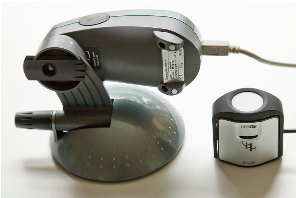
Figure 2.9: The X-Rite i1 colorimeter for measuring colors of displays.
