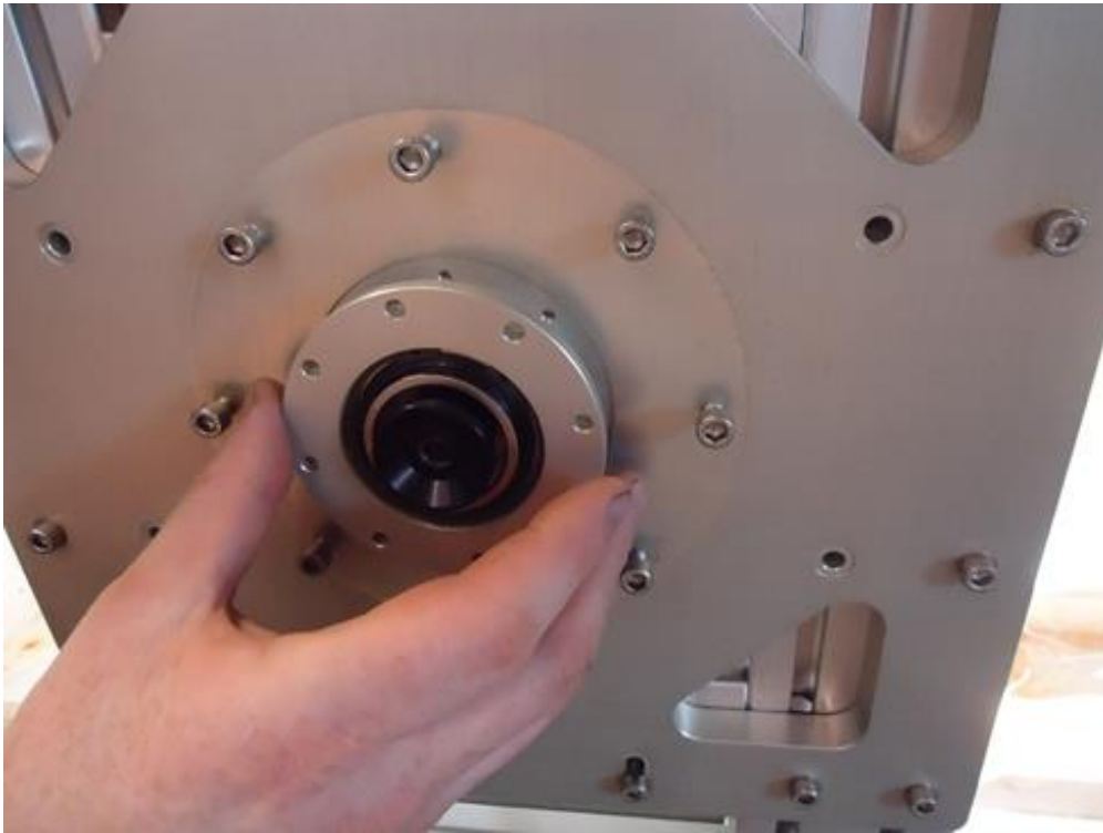
Figure 19: Mounting the bearing outside the camera support
