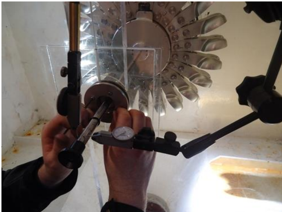
Figure 17: Final balancing of the 90° angular adapter
