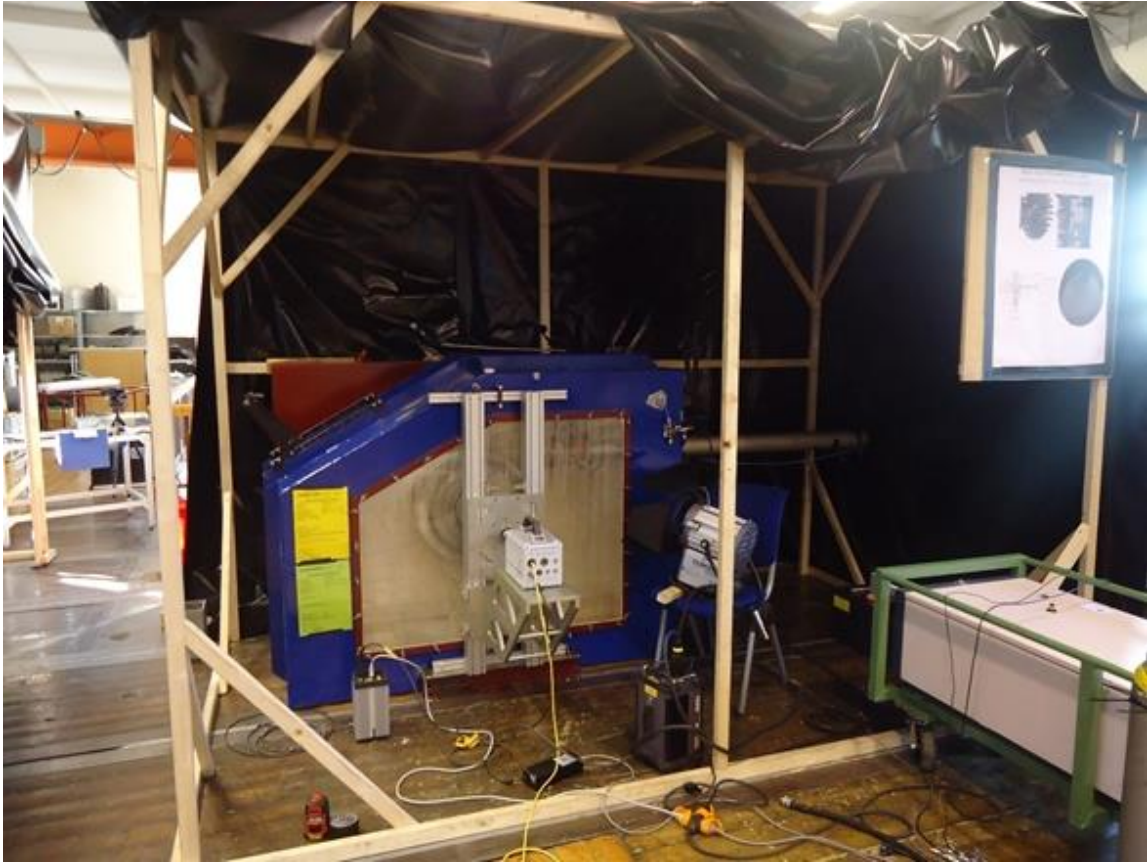
Figure 7: Complete installation, with the laser for lighting placed to the right. The other light sources are only used during installation
