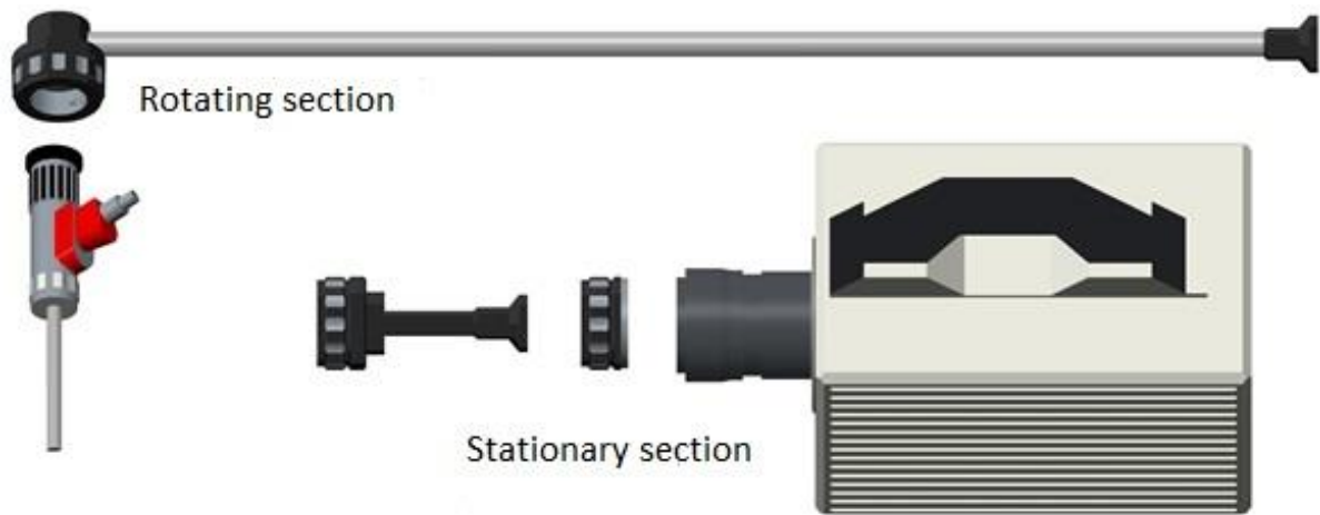
Figure 5: The optical system is split in a rotating and a stationary section
