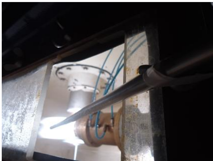
Figure 9.4: One optical fiber-cable for laser light placed inside a metal pipe, situated just over the nozzle exit.
