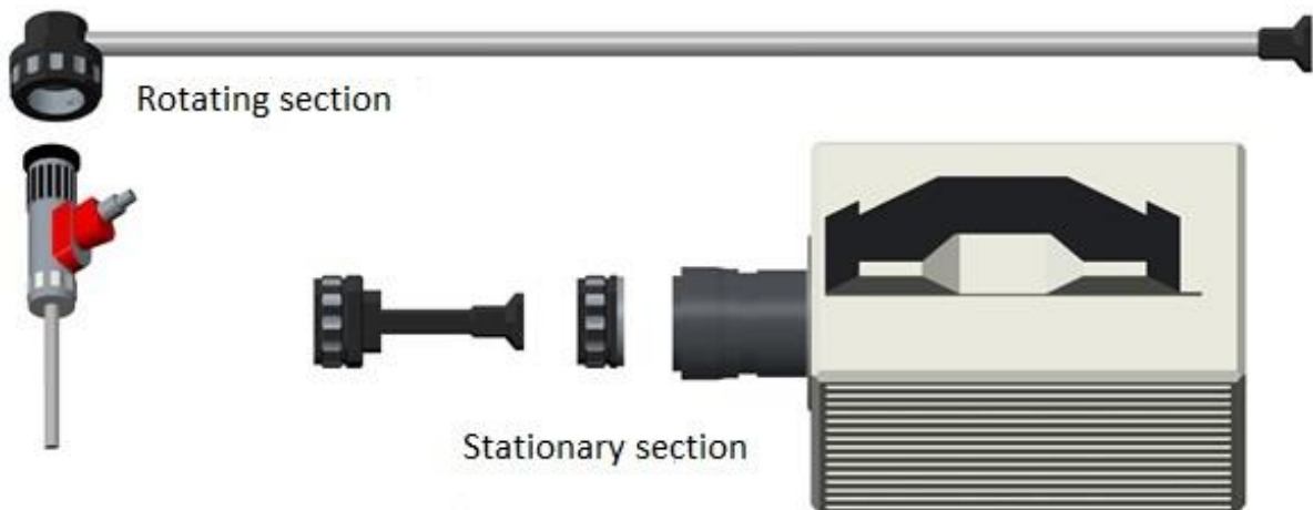
Figure 8.5: The optical system is split in a rotating and a stationary section
