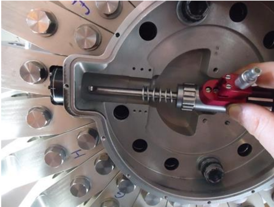
Figure 12: The placement of the borescope
