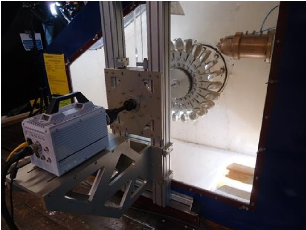
Figure 20: Aligning the camera with the adapter, while fastening it to the support
