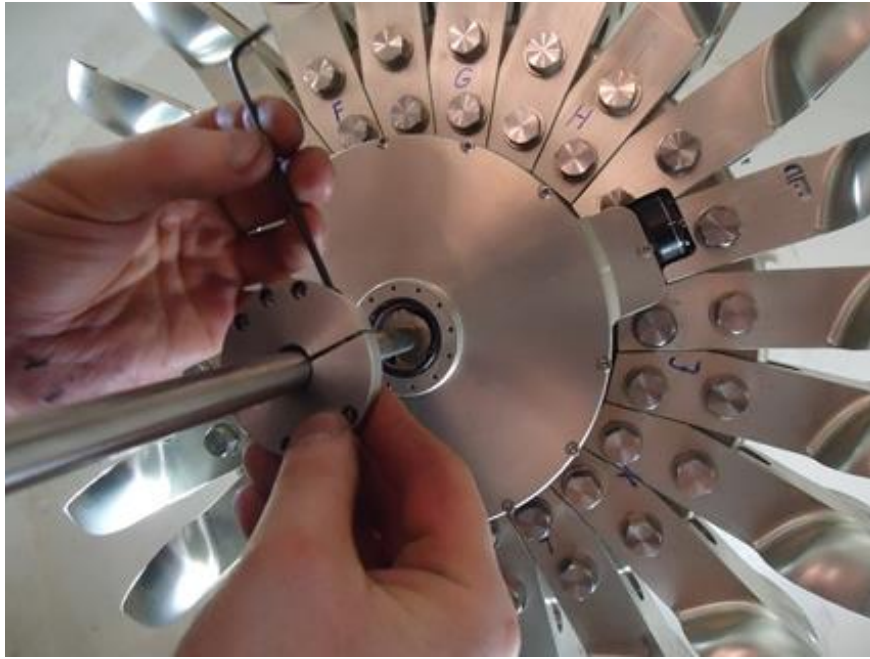
Figure 15: Fastening the cover of the borescope casing
