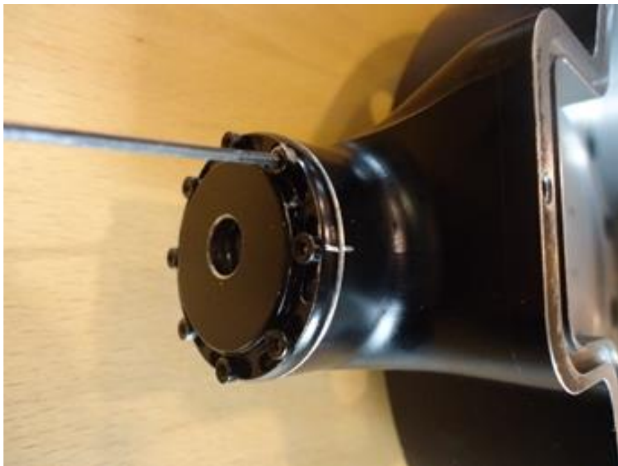
Figure 10: Fastening the lid for the borescope casing. White marks indicate the right position
