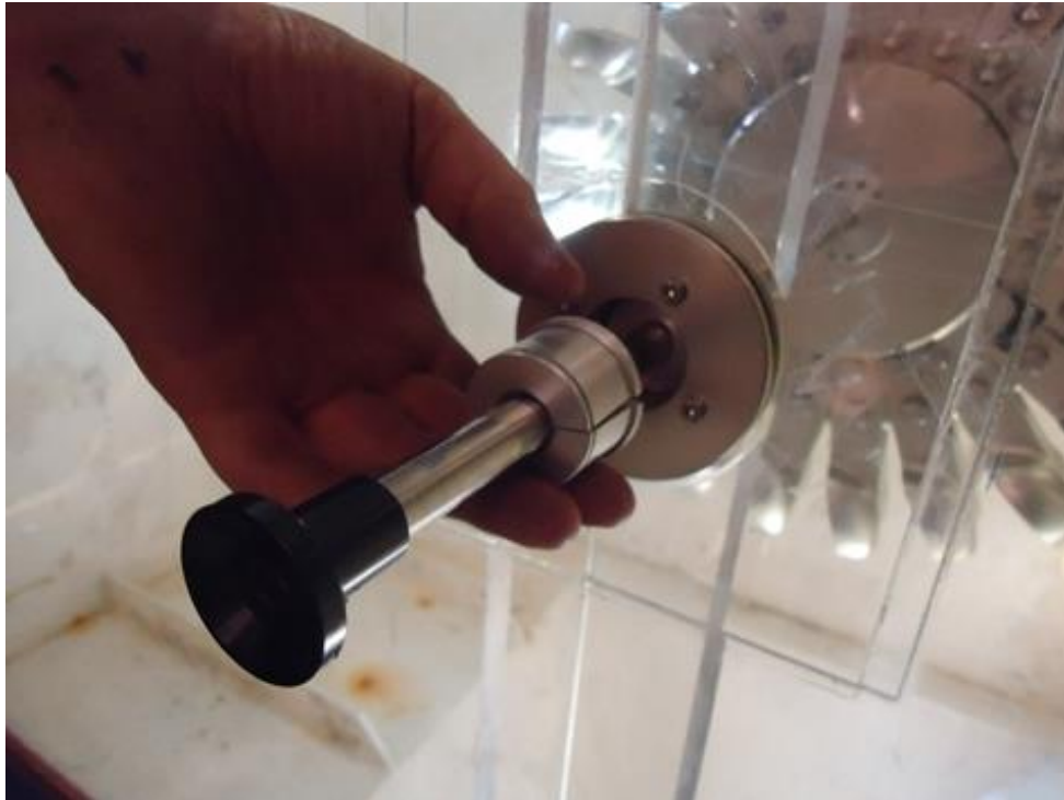
Figure 18: Fastening the clamp to lay inside the bearing in the camera support
