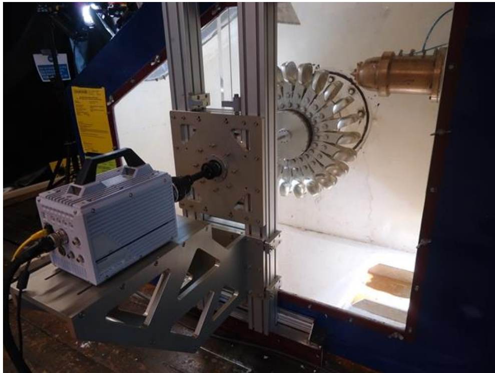
Figure 9.1: Installed new setup, with an onboard borescope
