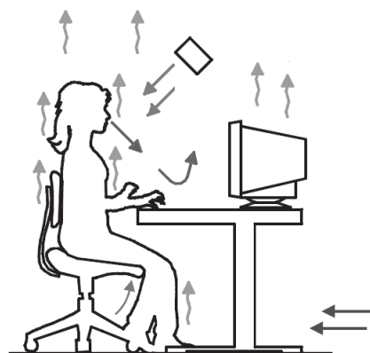
Figure 7.19: Illustration of personal ventilation at a work desk. Figure: (Melikov, 2004)
