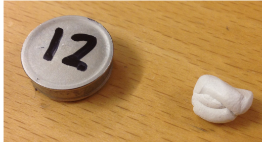
Figure B.2: The iButton sensor and the pressure sensitive adhesive used to attach it to various surfaces.
