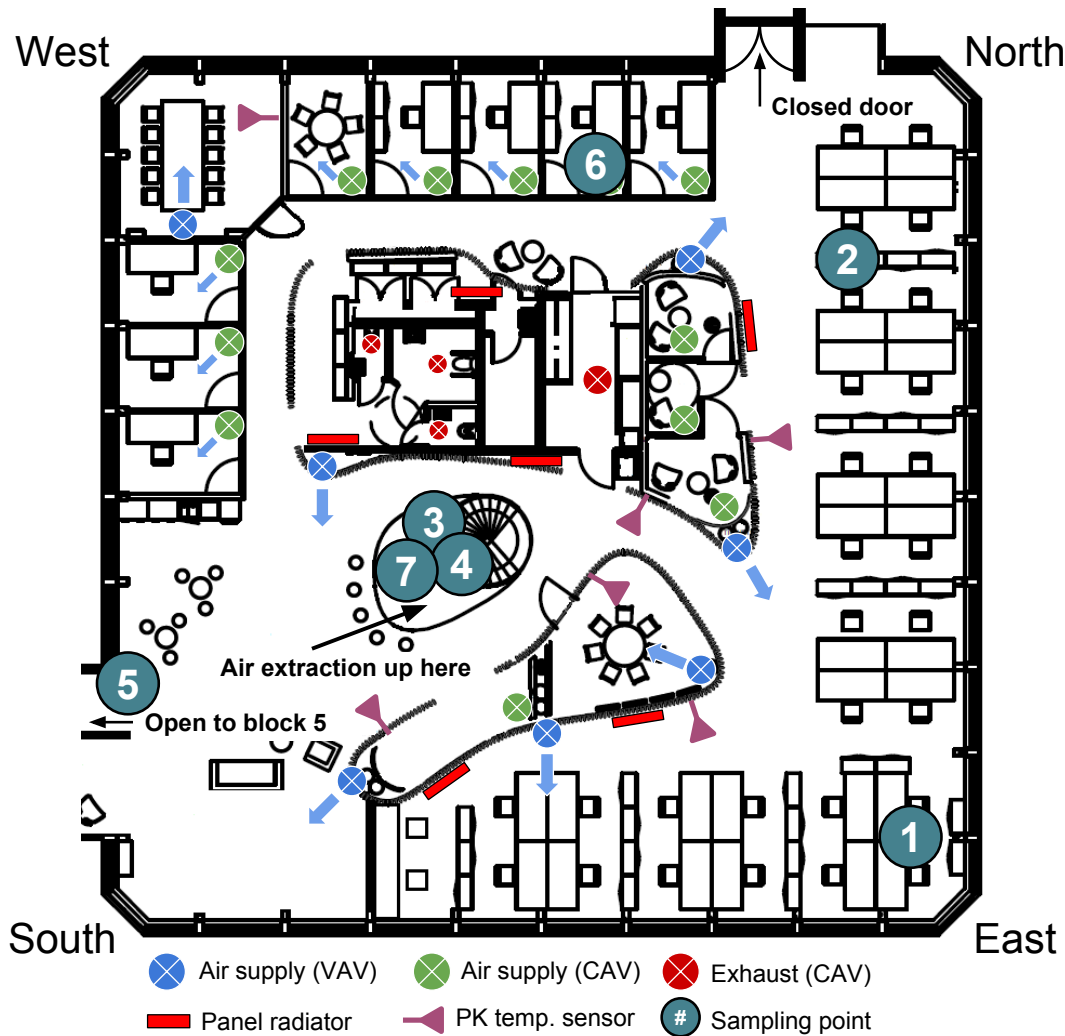
Figure 6.3: The locations of the sampling points during the ventilation efficiency experiment at the 2 nd floor, block 4. Sampling point 4 and 7 is at the 3 rd and 4 th floor respectively. The exhaust points are for wet rooms and a printer room. The main exhaust (VAV) is up the staircase in the center. Technical drawing: Entra.
