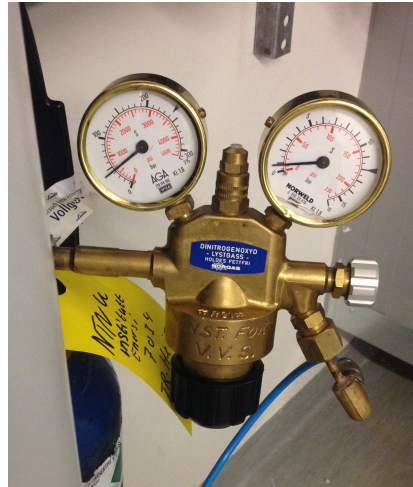
Figure A.5: Picture of the pressure control valve used at Powerhouse Kjørbo. It shows the inlet pressure from the bottle (left gauge) and the outlet pressure for the gas flow through the plastic tube (right gauge). Photo: Odin Søgner.
