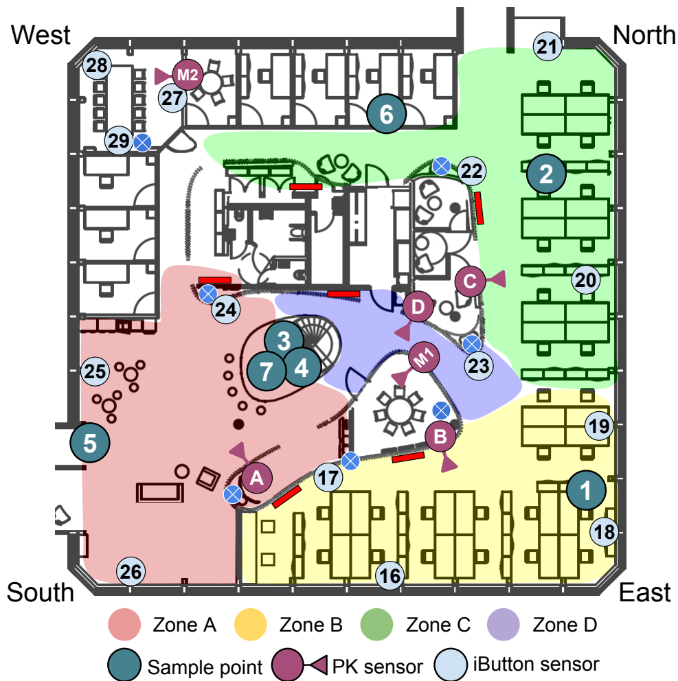
Figure 7.2: Division of zones on the 2 nd floor of block 4. The iButton and PK temperature sensors, and the tracer-gas sample points are included in the figure ( Technical drawing: Entra ).
