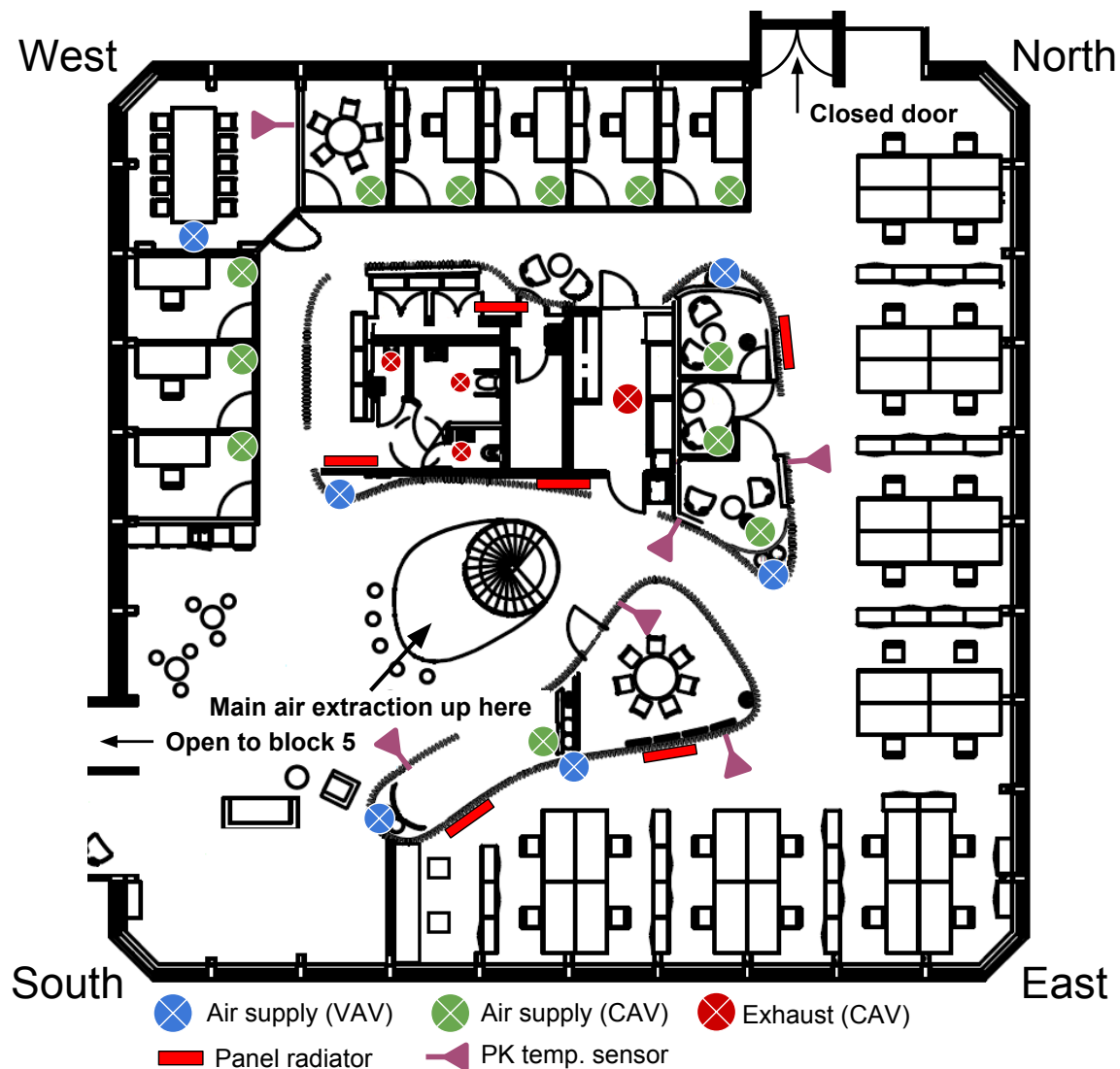
Figure 4.7: Building plan of the 2 nd floor in block 4. It illustrates the placement of the permanent temperature sensors, the air diffusers and ventilation strategy and the radiators. Technical drawing: Entra.
