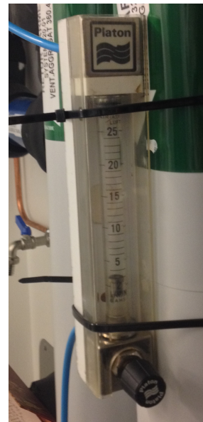
Figure A.6: Picture of the rotameter used at Powerhouse Kjørbo. The nitrous oxide is supplied at the bottom, through the conical tube and exits at the top. Photo: Odin Søgner.
