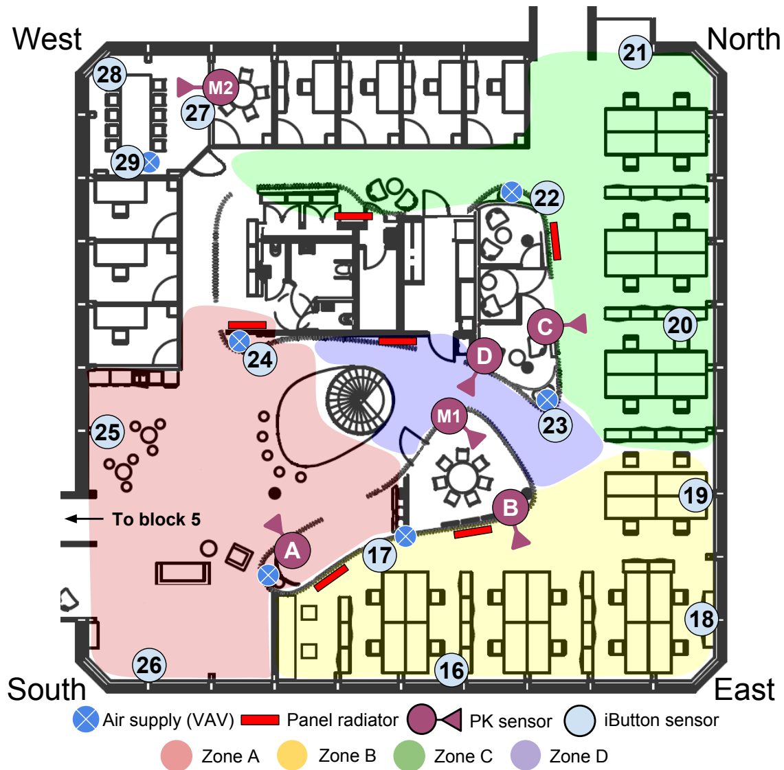
Figure 6.1: Illustration of sensor positions at 2 nd floor, block 4. Each zone is marked with its distinct color and is named after the PK sensor in its area. Technical drawing: Entra.
