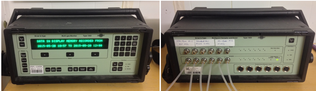
Figure A.4: Brüel & Kjær Multi-gas Monitor - Type 1302 (left) and Multipoint Sampler and Doser - Type 1303 (right). Picture: Odin Søgne
