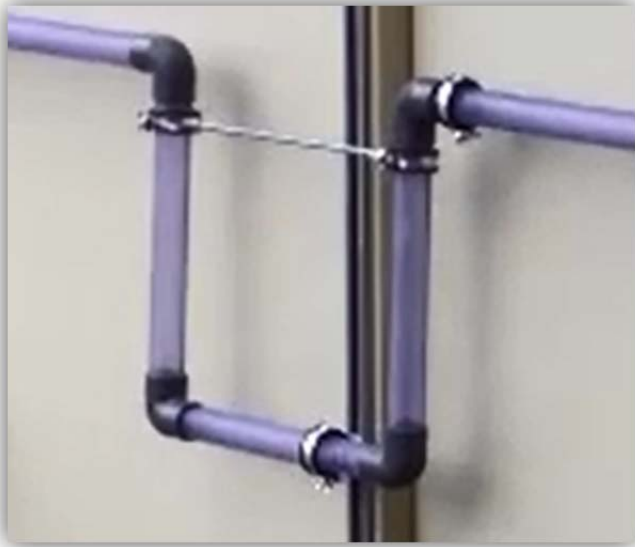
Figure 3: No trace of stocked frost formation in the pipes after relief of PRV.
