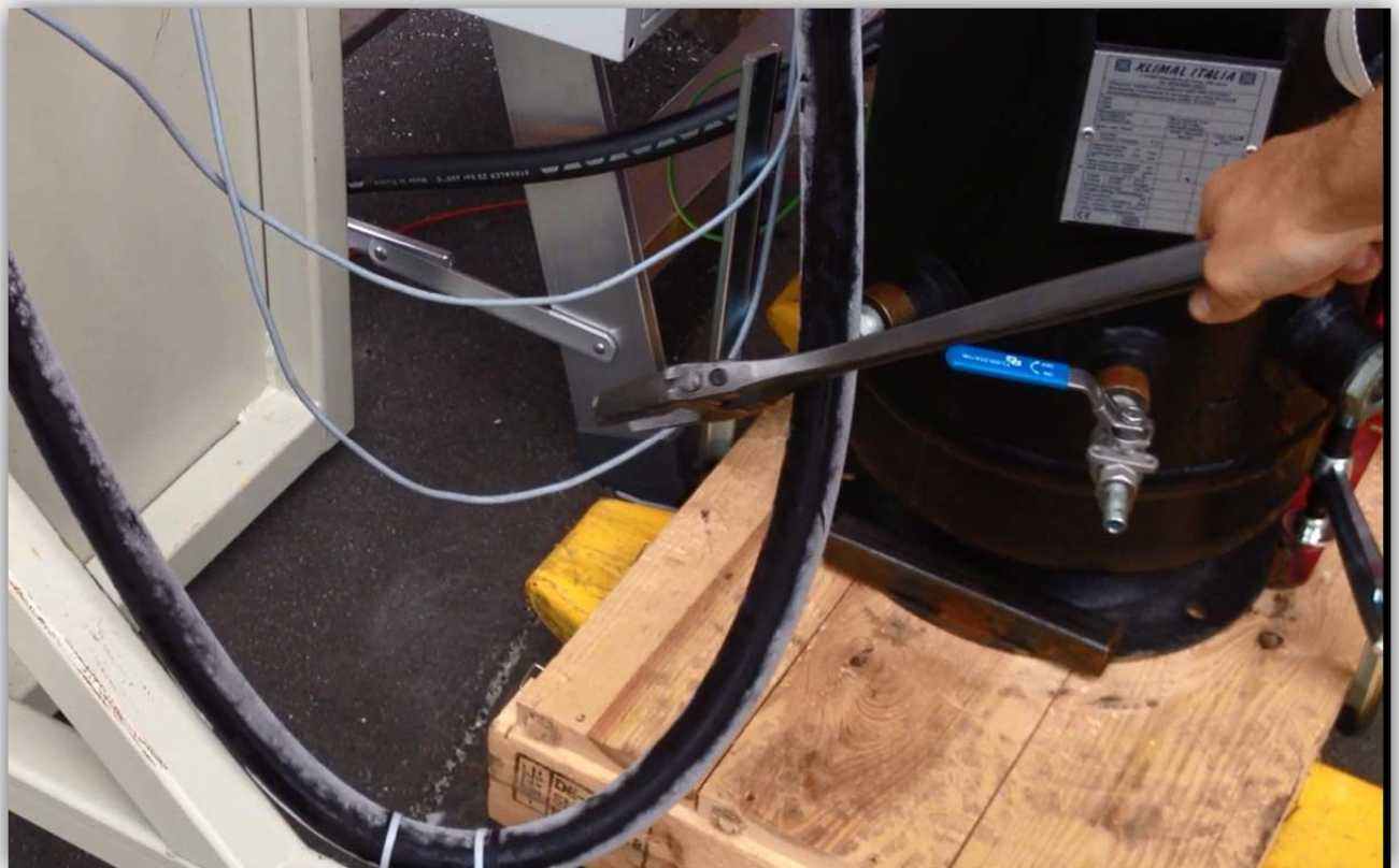
Figure 4: Hose is still flexible after relief of PRV and not fragile.
