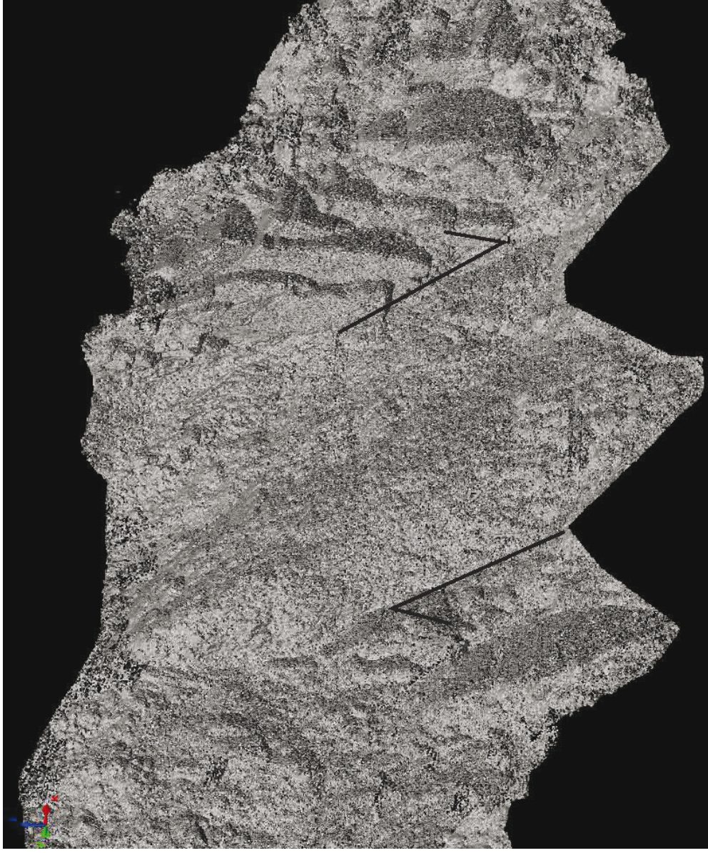
Figure 4-14: LIDAR model of locality 2) Rød, here shown by the point cloud. Arrows indicate relative movement of the most recent event of faulting.
