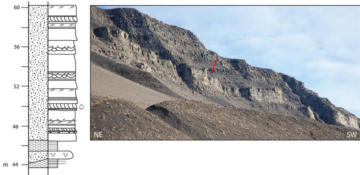
Figure 46: Channels on Siegfjället. Lateral continuous for kilometers. Profile measured summer 2008 by Glørstad-Clark. See Appendix 8 for panorama of Siegfjället.
