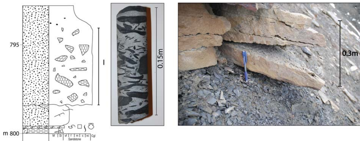
Figure 28: Mud flake conglomerate in core interval B (see Appendix 4) and in section BOT093 (see Figure 5) on Botneheia. The mud flakes are from a few mm up to about 6 cm, and some are clearly deformed in the core material.
