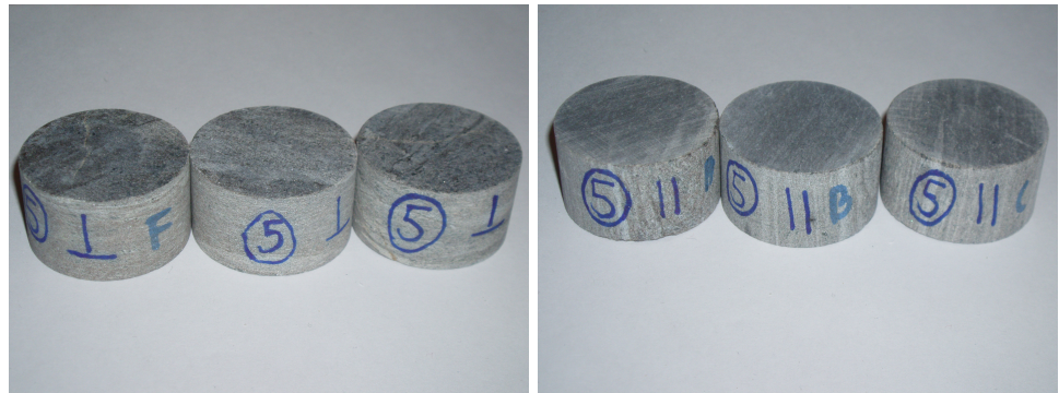
Figure E.8: Core sample 5. Normal orientation on the left and parallel orientation on the right. Photo: Marie Stølen
