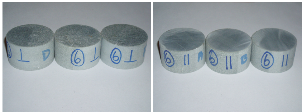
Figure E.9: Core sample 6. Normal orientation on the left and parallel orientation on the right. Photo: Marie Stølen
