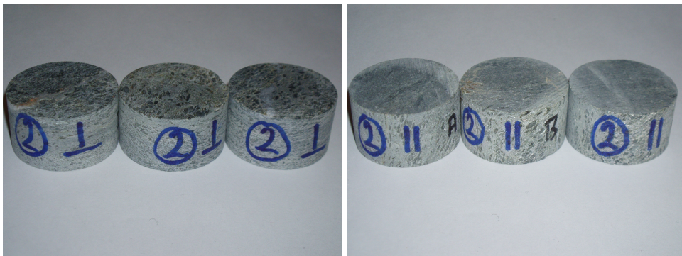
Figure E.5: Core sample 2. Normal orientation on the left and parallel orientation on the right. Photo: Marie Stølen
