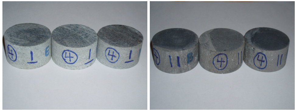
Figure E.7: Core sample 4. Normal orientation on the left and parallel orientation on the right. Photo: Marie Stølen
