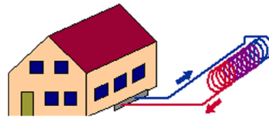
Figure 2.9: Spiral-type ground heat exchanger (Sanner, 2001)
