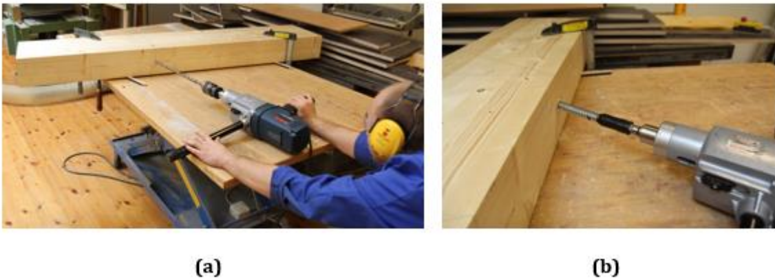
Figur 3.6 (a) forboring (b) innskruing.
