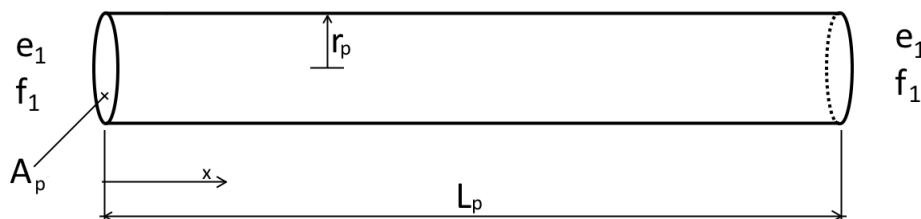
FIGURE 5.2: Fluid transmission line. Uniform cross sectional area A_p , length L_p radius r_p
