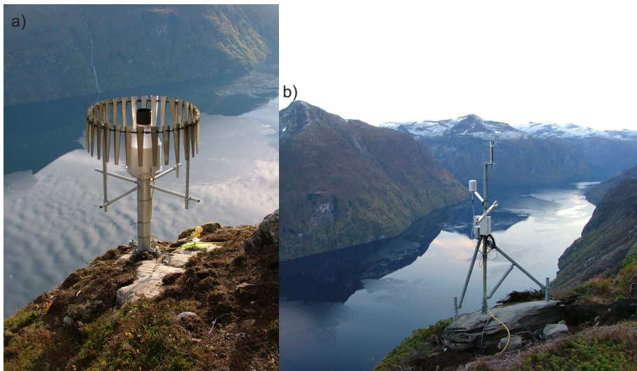
Fig. 3 Meteorological station at Åknes at 900 m a.s.l. operational from 11 November 2004. a) Precipitation gauge (Oscillating string T-200 B from Geonor) b) Meteorological mast monitoring air temp/humidity (Combinationsensor HMP45A from Vaisala), soil temperature (Thermistor 107 from Campbell), wind speed/direction (Windobserver II from GILL), radiation (Combinationsensor CNR1 from Kipp&Zonen), and snow depth (Ultrasoundsensor SR50 from Campbell). The measuring frequency is 5 sec for all instruments except for the snow depth sensor, for which it is 15 min.
