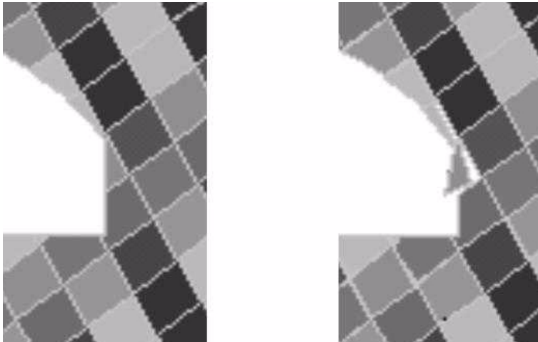
FIGURE 5.19 Block movements Model 4, varying Poisson's ratio left \nu = 0,2 and right \nu = 0
