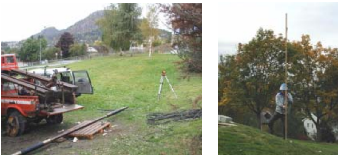
Figure 4–20: The levelling set up at EAB. Levelling telescope and levelling staff.
