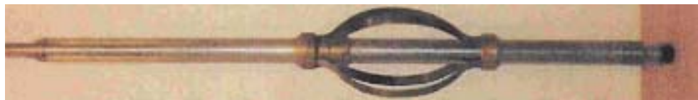
Figure 2–19: Impeller flow meter probe (Elvebakk and Rønning, 2003).
