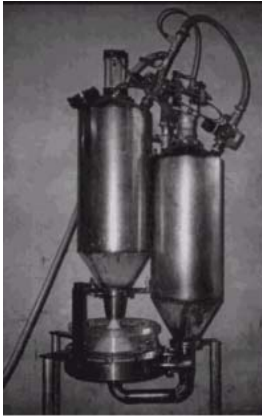
Figure 2–15: Air pressure mixer for the mixing and rapid hydration of thickener and water.
