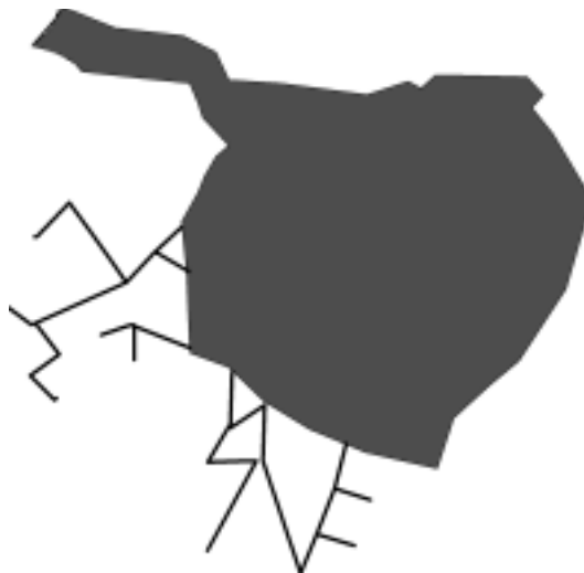
Figure 4–24: This is how fractures can be designed in FEFLOW. The black lines represents fracture channels, while the black area is a fracture plane (Spangelo, 2002).
