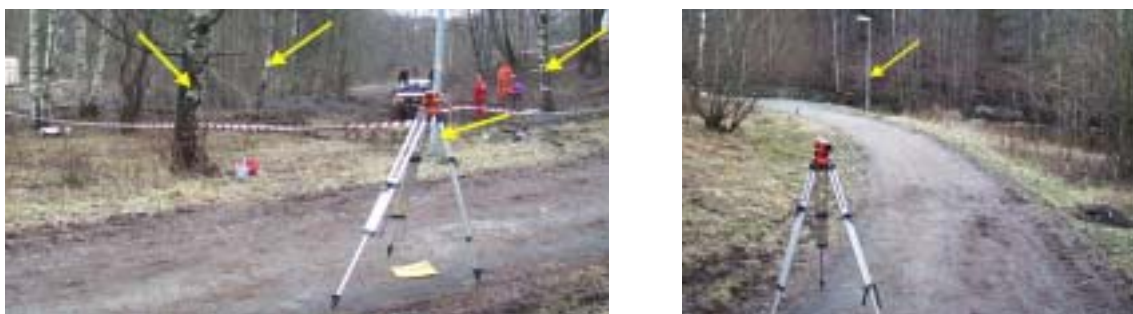
Figure 4–13: A general overview of the levelling points within the area of assumed influence for hydraulic fracturing (left), and the fixed point (right). The pictures at Bryn are turned 180° with respect to each other.
