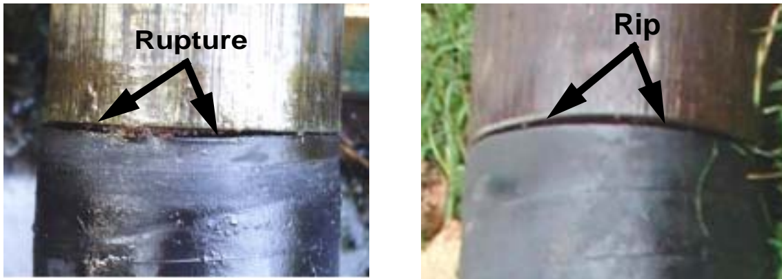
Figur 5–98: Blown lower packer element from the hydraulic fracturing with water-only in borehole 2 at Bryn (left), and a rip on the packer element from the hydraulic fracturing with injection of sand in borehole 2 at EAB (right).
