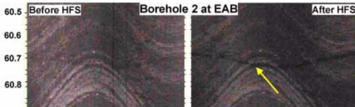
Figure 5–70: A segment of borehole 2, recorded with an optical televiewer before and after hydraulic fracturing with injection of sand. The existing fracture at 60.7 metres is clearly more open after the hydraulic fracturing with injection of sand.
