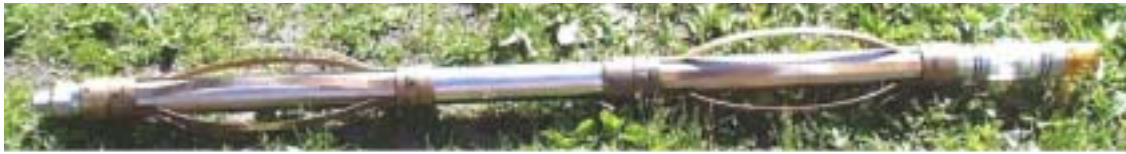
Figure 2–16: Probe for optical televiewer inspection of boreholes equipped with centralizers. Video camera unit at the right.
