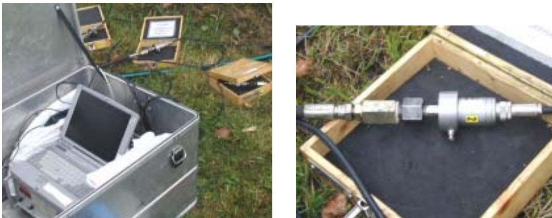
Figure 2–12: At left: Pressure sensors connected to a measuring bridge, which is connected to a data logger. The recorded data are loaded into a laptop. At right: A pressure sensor.
