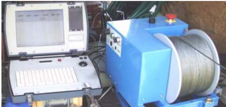
Figure 2–17: Computer controller and cable reel for optical televiewer.
