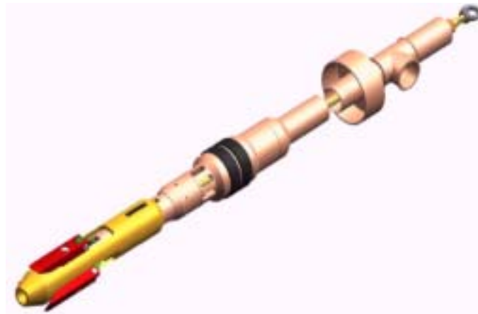
Figure 2–14: Injection packer for the re-injection of groundwater into the central borehole at Bryn.
