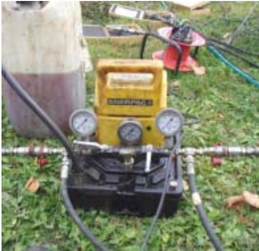
Figure 2–8: A small high-pressure oil pump for the pressurization of upper and lower packer on FrakPak - AIP 410-550 using a low viscosity oil. In front: Two ports for the measurement of the packer pressures.
