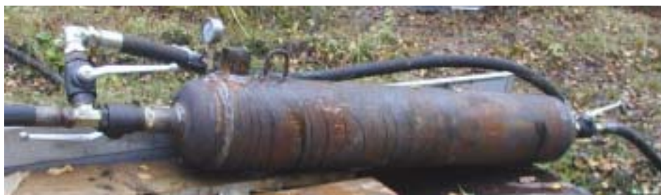
Figure 2–13: A high-pressure tank for storage of the injection fluid used in the procedure for hydraulic fracturing with injection of sand.
