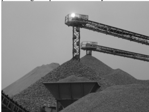
Figure 4: Example of tool for reducing height of fall for quartz raw materials.
