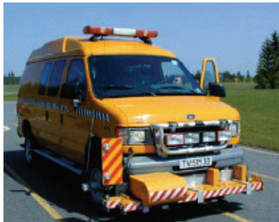
Figure 4-20. ALFRED rut measurement device mounted in front of vehicle (Photo by Statens vegvesen)
