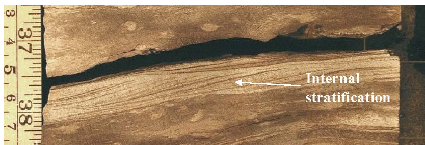
FIGURE 5.29 Core photo of the interval between 2604.93-2604.98 showing a sand laminaset with internal stratification resembling the Type II ripple.
