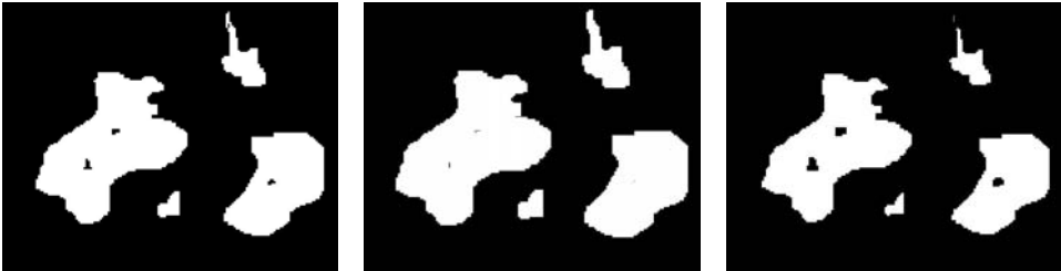
Figure 5-3. Original binary image (left), three cycles of dilation of the original image (middle) and 3 cycles of erosion of the original image (right).
