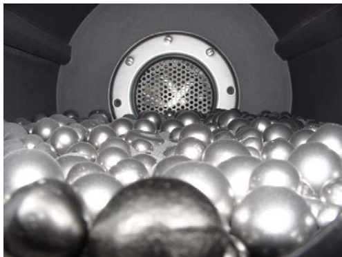
Figure 2. Picture showing the inside of the mill.
