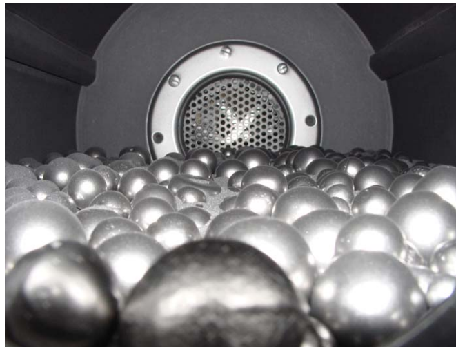
Figure 4.5 The inside of the ball mill.
