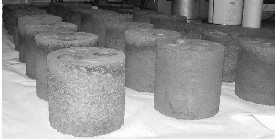
Figure 6.16 Photograph of the baked anodes.
