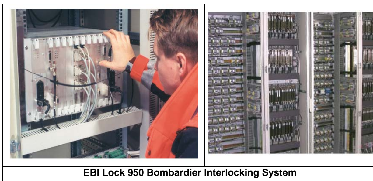
Figure 9 EBI Lock 950 Bombardier Interlocking System
