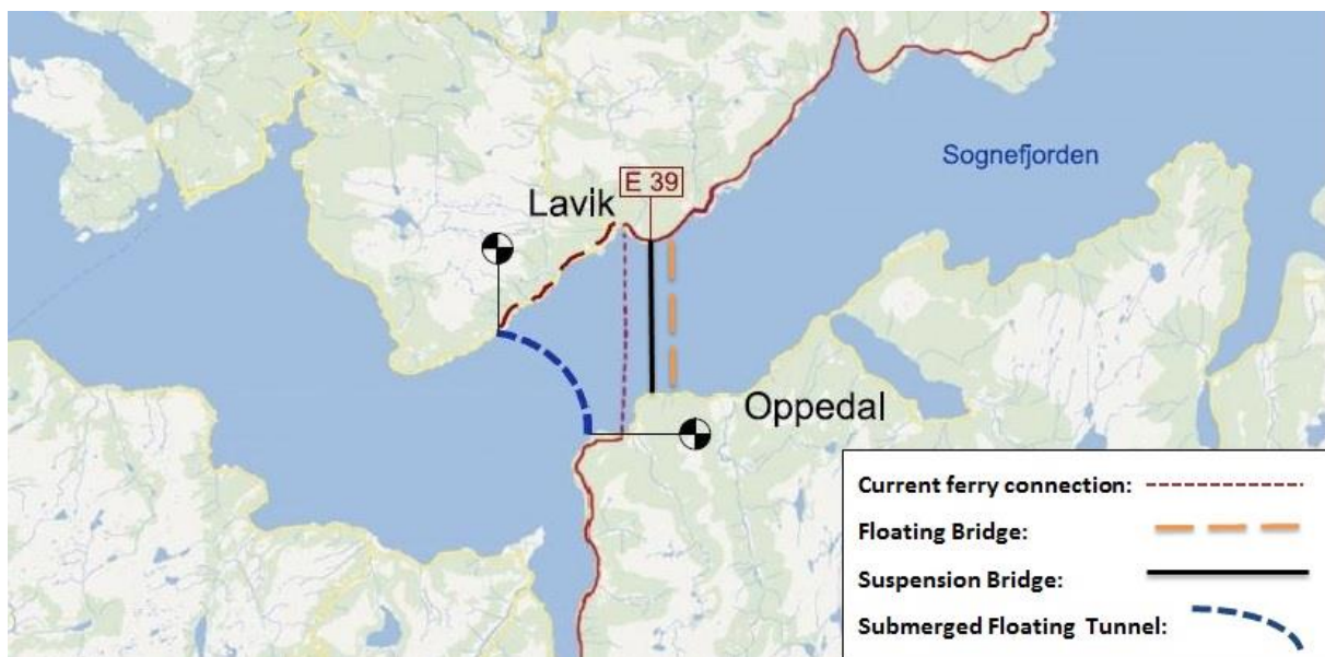
Figure 5: The current ferry connection and proposed site for crossing the Sognefjord modified from Fjeld (2012). The figure was made for illustration purposes, and exact bridge location may not be accurate.
