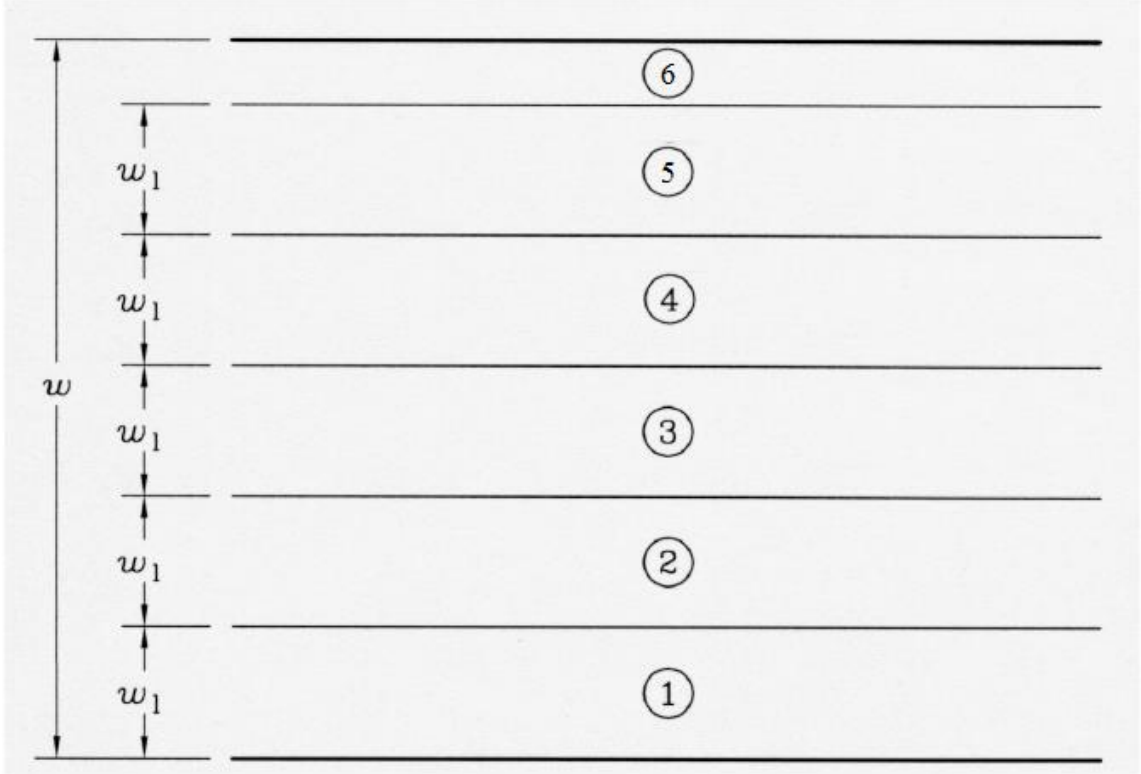
Figure 5.1: The total carriageway width of Elgeseter Bridge results in five notional lanes, and a remaining area, 6.
