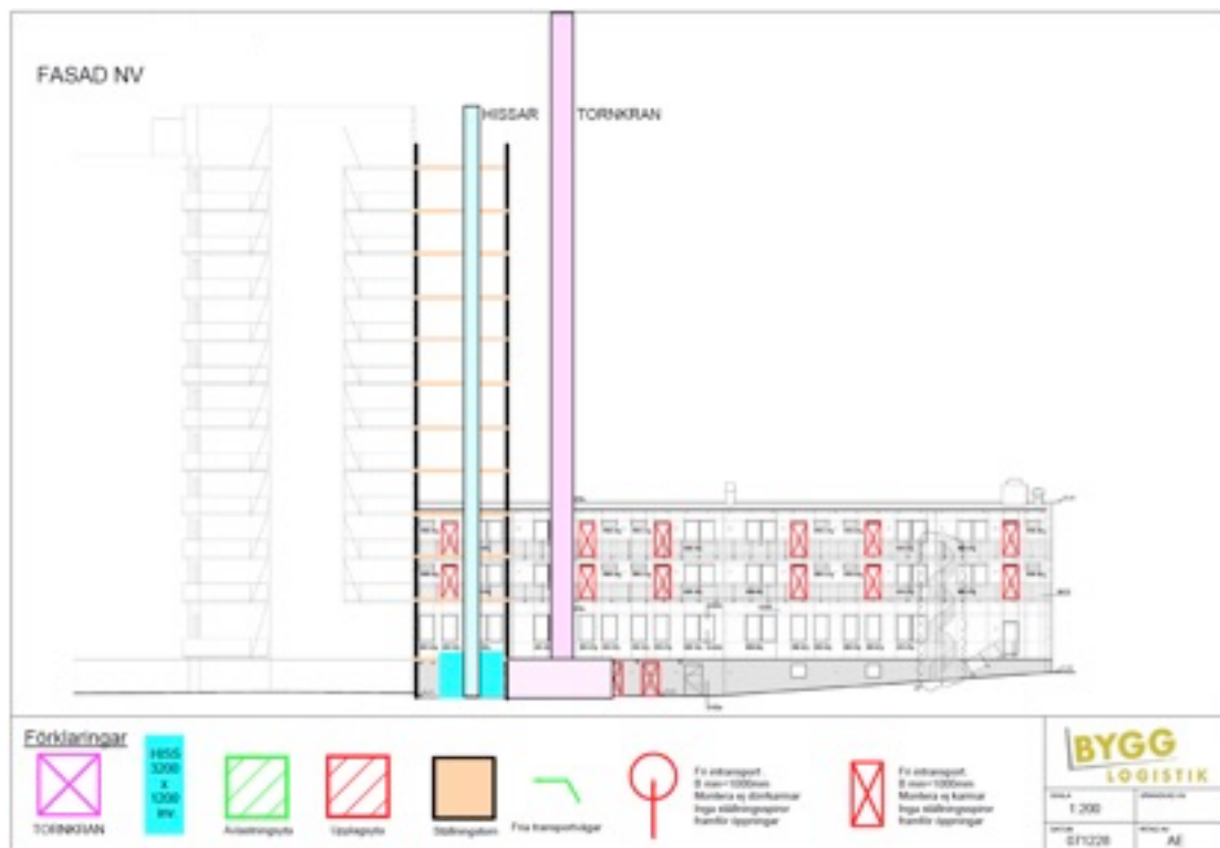
Figure 22 Temporary openings for materials
