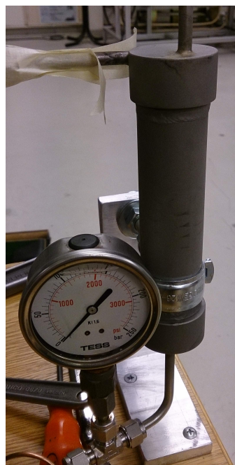
Figure 18: Separation tank after installation
