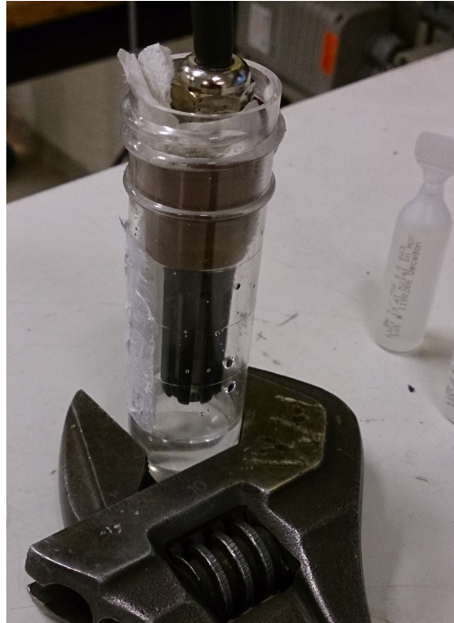
Figure 26: Humidity calibration setup
