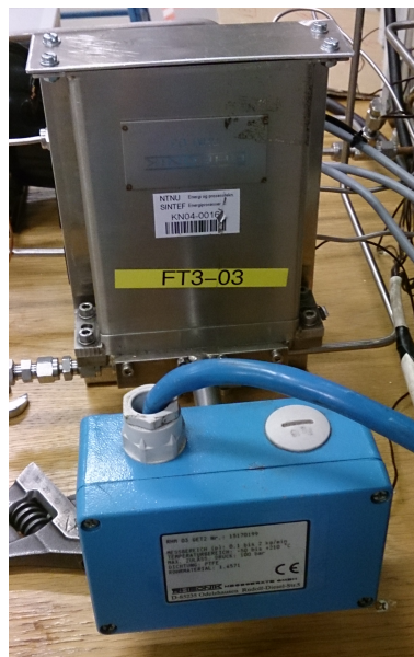
Figure 22: Rheonik RHM 03 mass flow meter
