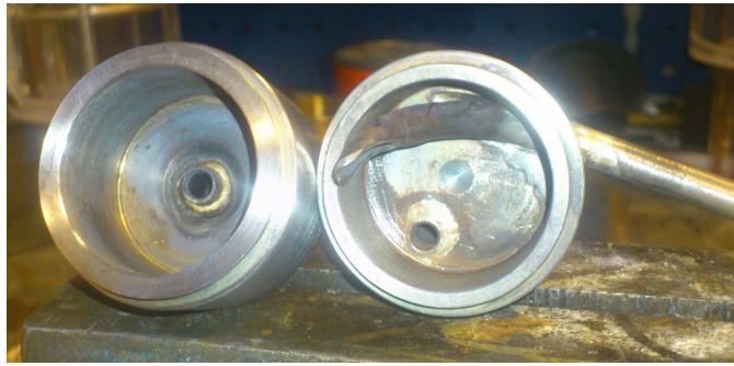
Figure 16: Internal view of the separation tank
