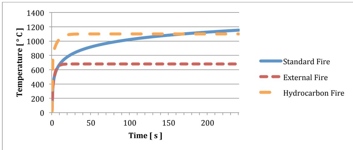
Figure 3-6 Nominal temperature-time curves given by NS-EN 1991-1-2 (Norsk Standard, 2008)
