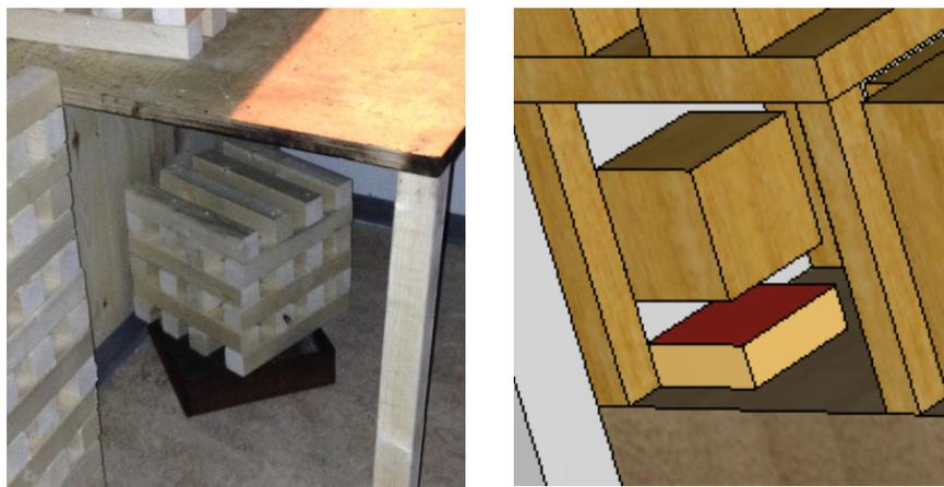
**Figure 6-11 Positioning of heptane burner in experiment and heptane burner drawn as “Block Obstruction” in PyroSim**
