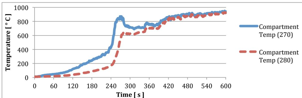
**Figure 6-6 Temperature measured in the compartment in the conducted experiment 270 cm and 280 cm above the floor**
