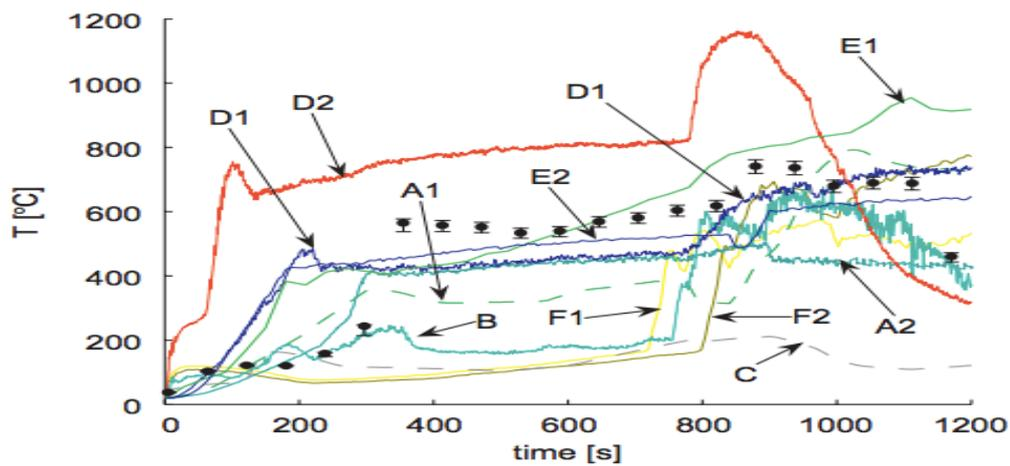
**Figure 5-2** Results gathered through simulations and observations conducted on the Dalmarnok Fire Test One. Evolution of the average temperature of the hot gas layer in the compartment. The black dotted line is the data conducted in the experiment, with error bars (Rein et al., 2009).
