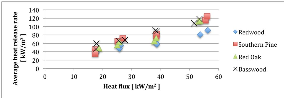
**Figure 4-10 Average heat release rate for various heat fluxes (Tran and White, 1992)**
