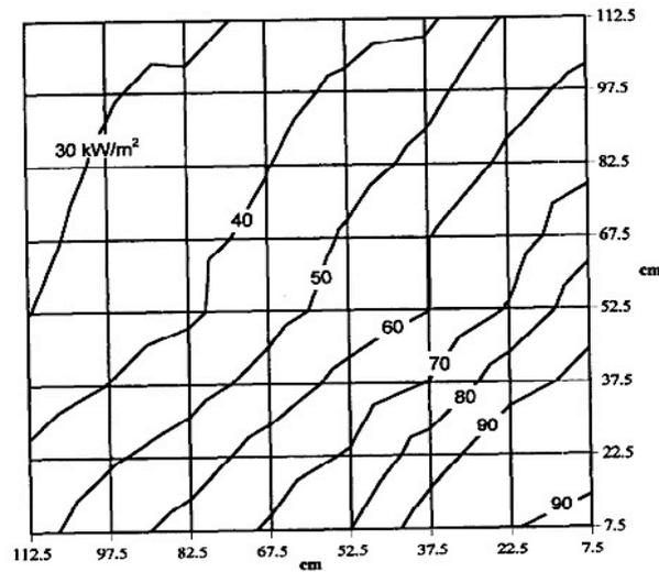
**Figure 4-14 Incident fire plume distribution to a cold ceiling. 0.17x0.17m square burner at 300kW, top surface 30cm from floor.**
