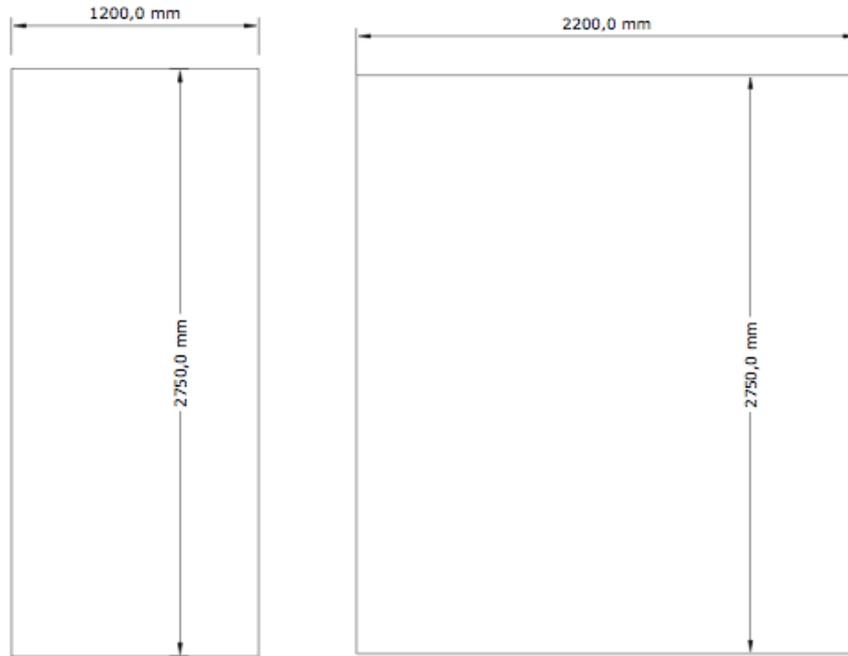
**Figure 6-3** Sketches presenting the measurements of height and width of the compartment used in calculations. Left sketch is the width in the entrance of the compartment, while right sketch is further in. The measures have been carried out manually and may deviate some from the original floor plan.
