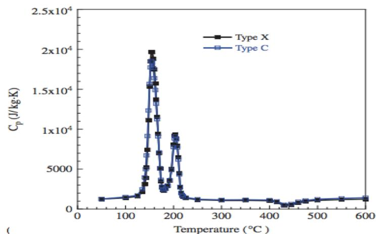
Figure 3-18 Specific heat of Type X and C gypsum plaster (Park et al., 2010)
