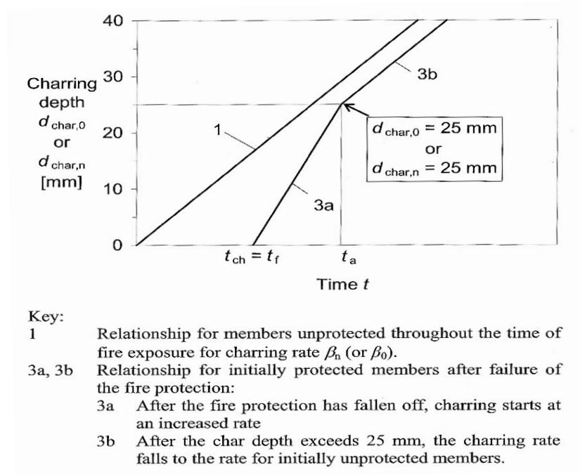
Figure 3-13 Variation of charring depth with time when  $t_{ch} = t_f$  and the charring depth at time  $t_a$  is at least 25 mm (Östman et al., 2010)
