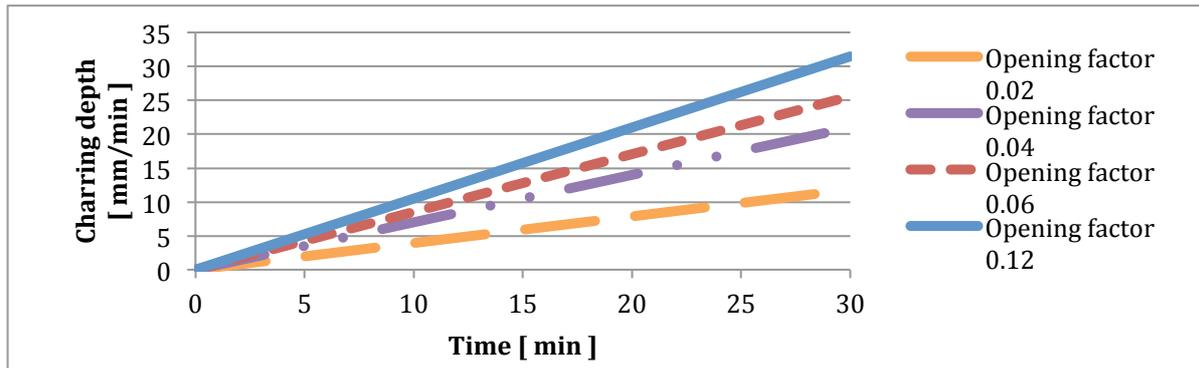
Figure 4-21 Char depth vs. time for varying opening factors, using the method presented in NS-EN1995-1-2 Annex A
