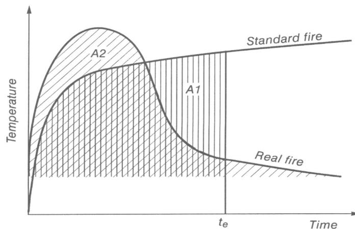
**Figure 4-2** Equivalent fire severity on equal area basis (Buchanan, 2002)
