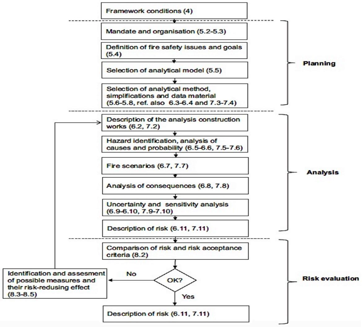
Figure 3-4 Flow diagram for risk assessments of fire in construction works (Norsk Standard, 2013)
