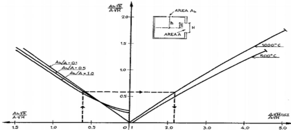
Figure 4-19 Graph for finding  $f_k$ , coefficient for calculating opening factor when a compartment has both horizontal and vertical openings (Magnusson and Thelandersson, 1970)
