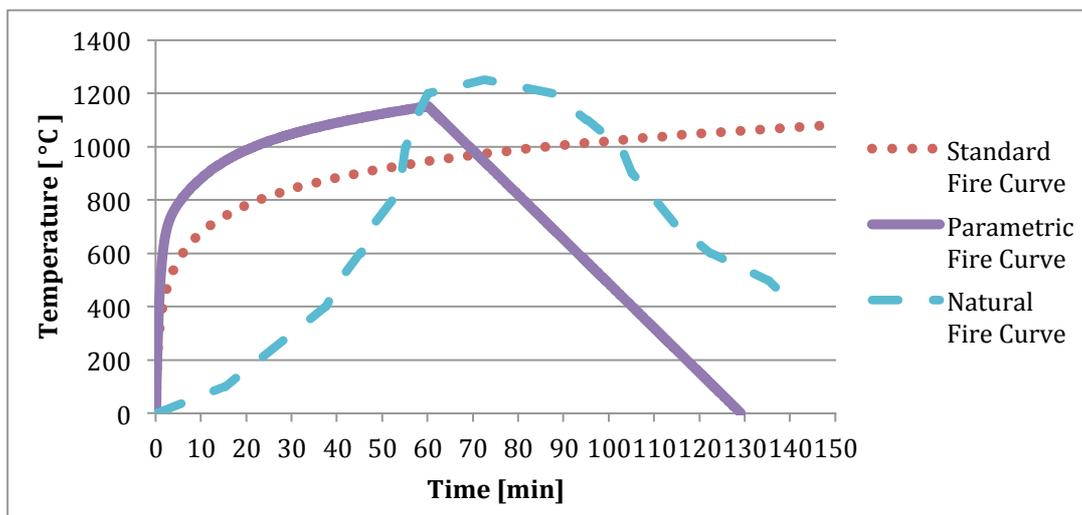
**Figure 4-1 Illustration of the two temperature-time curves presented in NS-EN 1991-1-2 and a assumed natural fire development**
