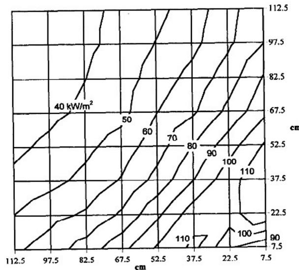
**Figure 4-15 Incident fire plume and room feedback heat flux distribution to a cold ceiling. 0.17x0.17m square burner at 300kW, to surface 30cm from floor.**
