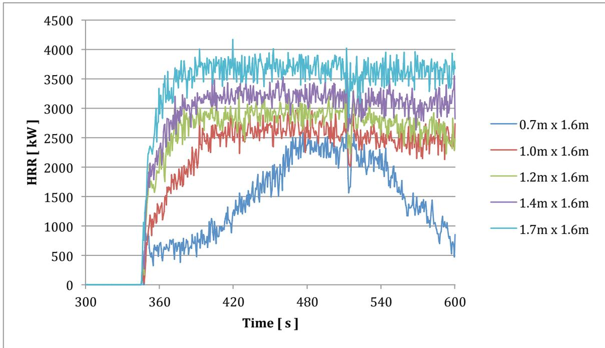
Figure 7-7 Heat release rate – time curves after the window breaks for the fire simulated in the compartment modelled.
