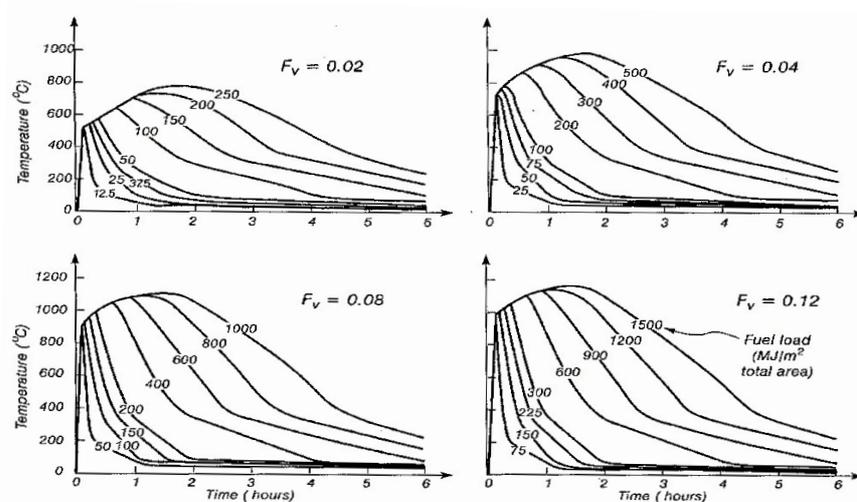
**Figure 3-8 Temperature-time curves for different ventilation factors and fuel loads (MJ/m<sup>2</sup> of total surface area), Swedish curves (Buchanan, 2002)**
