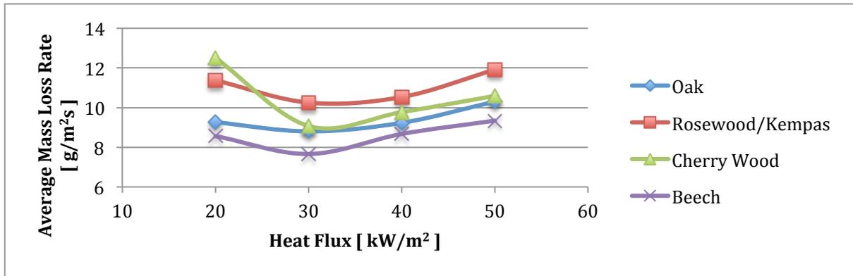
Figure 4-13 Average mass loss rate after ignition for various heat fluxes (Ji et al., 2003)
