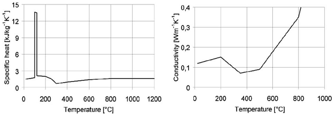
**Figure 3-10** The specific heat and conductivity of wood (Norsk Standard, 2010)
