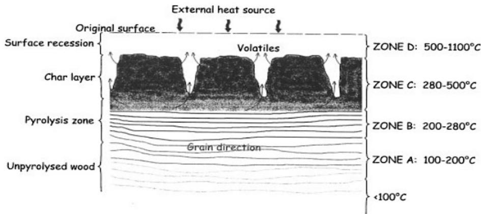
**Figure 3-9 Temperature zones in a solid wood cross-section exposed to fire (Friquin, 2011)**
