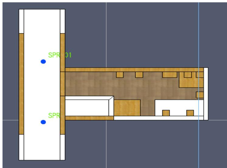
**Figure 6-8 Positioning of sprinkling system/nozzles**
