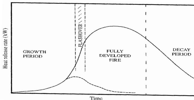
**Figure 3-5 Course of a well-ventilated compartment fire, expressed as the rate of heat release as a function of time**
