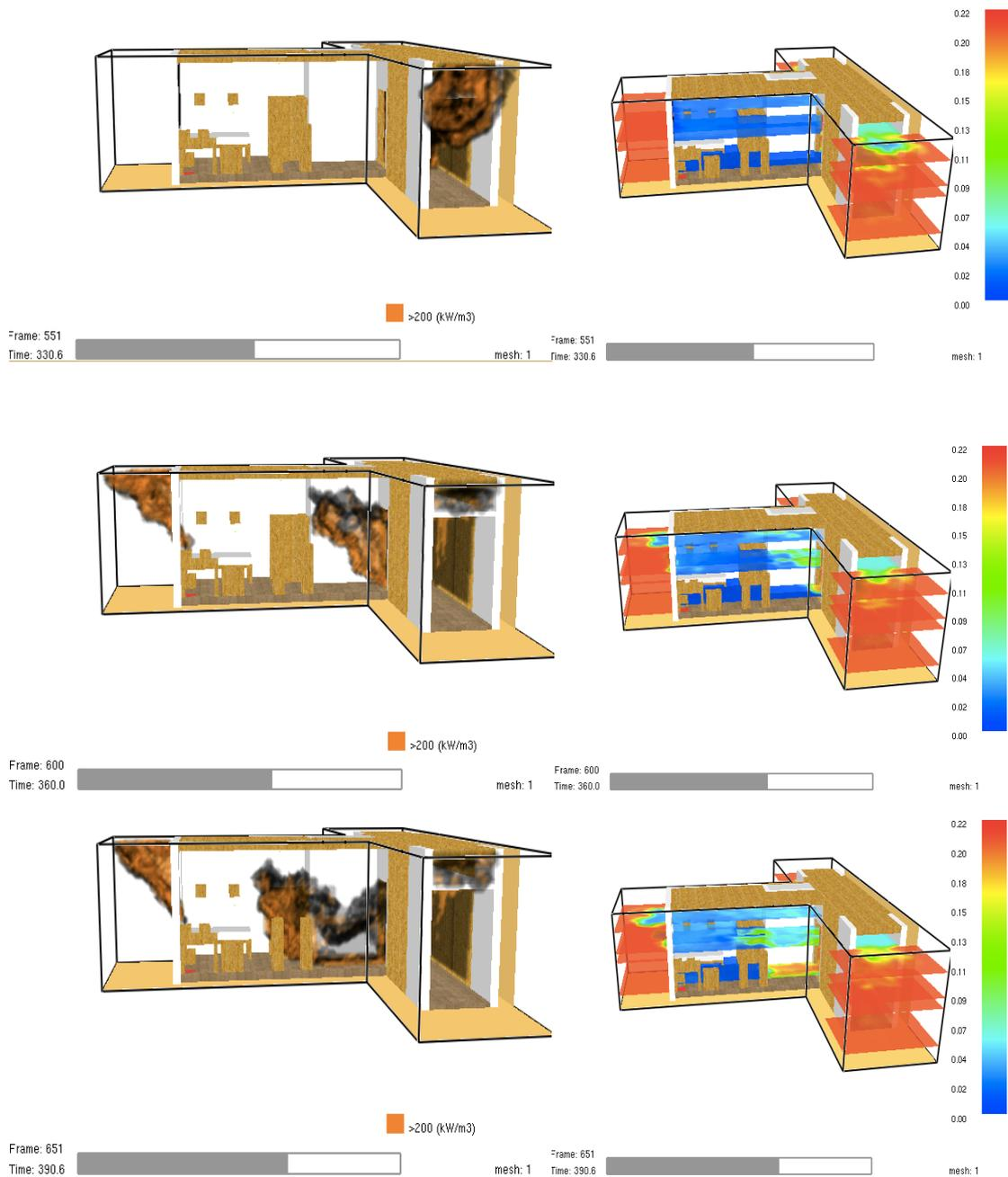
**Figure 7-4** The simulated fire behaviour 15 seconds prior to, 15 seconds after and 45 seconds after the window breaks, and the oxygen concentration in the compartment at the same time intervals. Window size: 1.2m x 1.6m.
