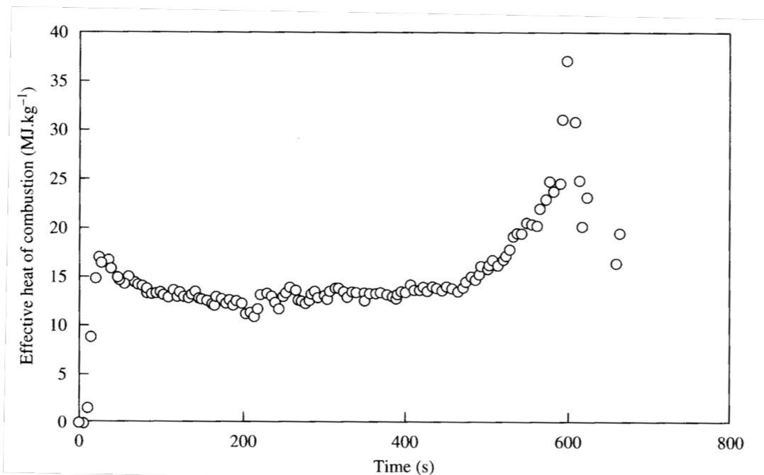
Figure 4-6 Instantaneous values of the effective heat of combustion of Western red cedar (17mm thick samples) at an imposed radiant heat flux of 65 kW/m<sup>2</sup> in the cone calorimeter, retrieved from: (Drysdale, 2011)
