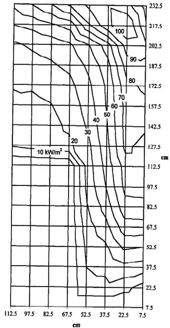
**Figure 4-16 Incident fire plume distribution to a cold wall. 0.17x0.17m square burner at 300kW, to surface 30cm from floor.**
