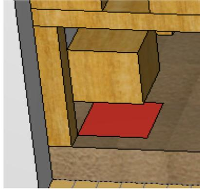
**Figure 6-12 Heptane burner drawn with "Vent" function in PyroSim**
