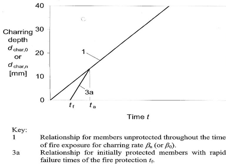
Figure 3-14 Variation of charring depth with time when  $t_{ch} = t_f$  and the charring depth at time  $t_a$  is less than 25 mm (Östman et al., 2010)
