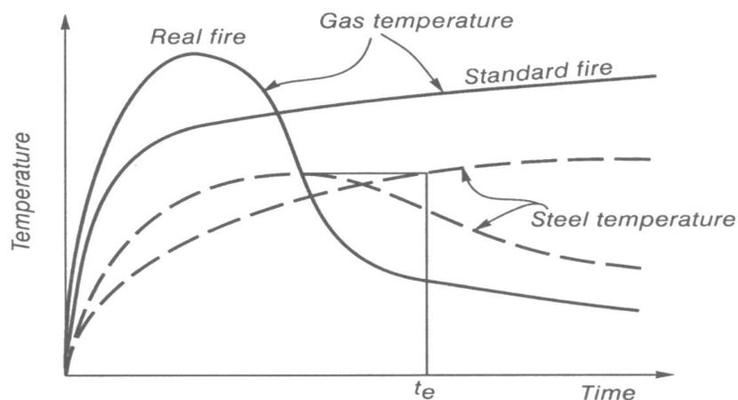
Figure 4-3 Equivalent fire severity on temperature basis (Buchanan, 2002)
