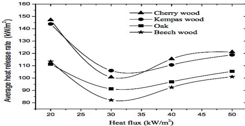
Figure 4-12 Average heat release rate of wood for varying heat flux. Retrieved from “The Pyrolysis and Heat Release Rate of Wood Exposed to Weak External Heat Flux for Long Times” (Chen *et al.*, 2004)
