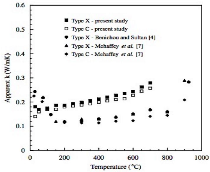
Figure 3-19 Thermal conductivity vs. temperature Type X and C gypsum plaster (Park et al., 2010)
