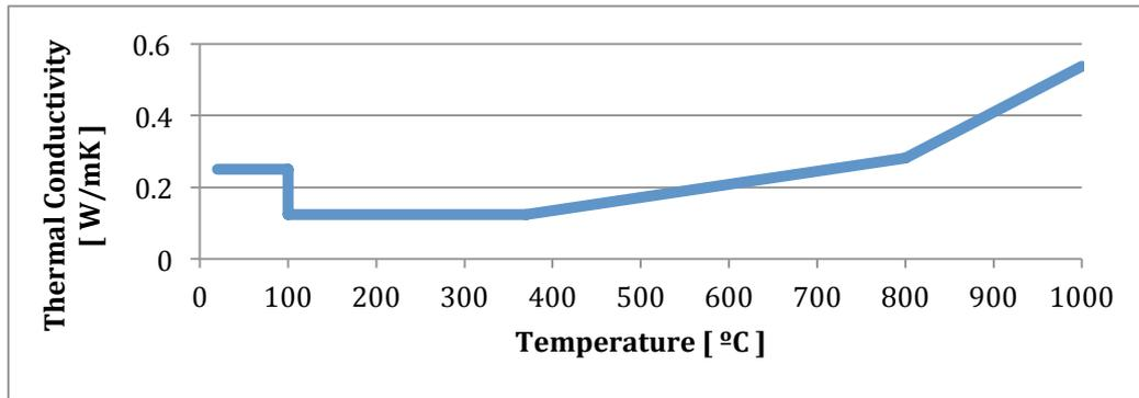
Figure 3-17 Thermal conductivity of gypsum plaster, for varying temperatures
