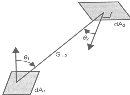
**Figure 4-8 Radiative heat transfer between two infinitesimal surface areas (Norsk Standard, 2008)**
