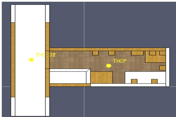
Figure 6-7 Positioning of thermocouples
