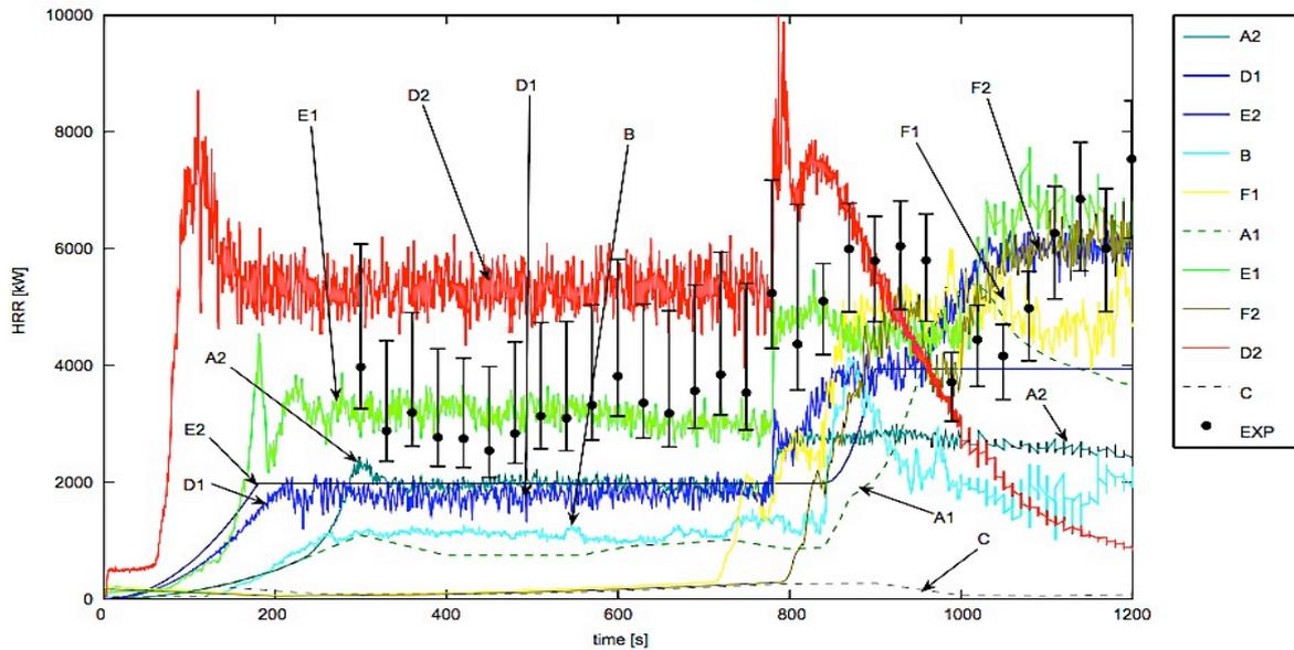
**Figure 5-1** Results gathered through simulations and observations conducted on the Dalmarnok Fire Test One. Evolution of the global heat release rate in the compartment. The black dotted line is the data conducted in the experiment, with error bars (Rein et al., 2009).
