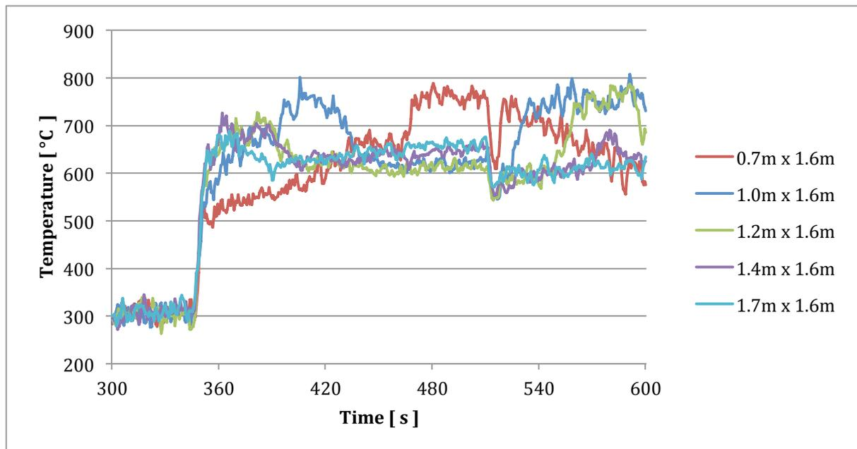
**Figure 7-6 Temperature – time curves after the window breaks for the fire simulated in the compartment modelled.**
