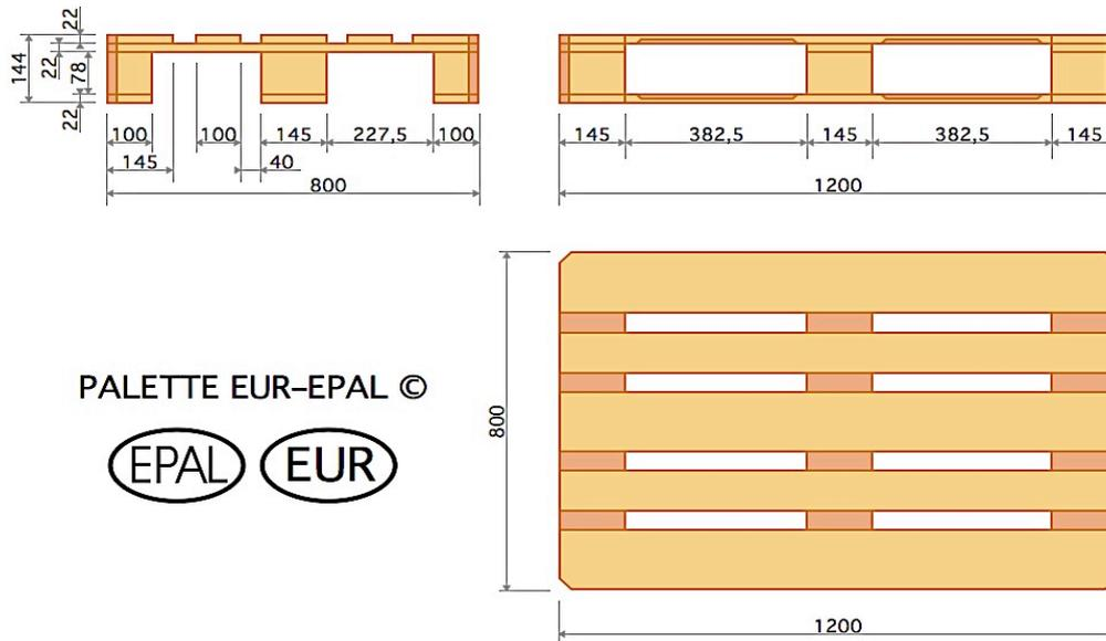
**Figure 6-9** Measurements of a standard Euro pallet
