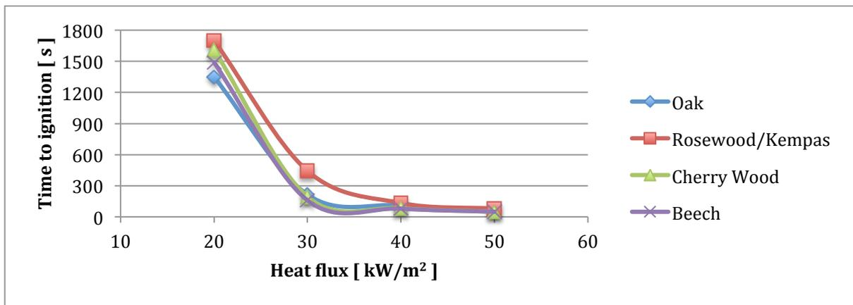
Figure 4-9 Ignition time for varying heat flux (Chen et al., 2004)
