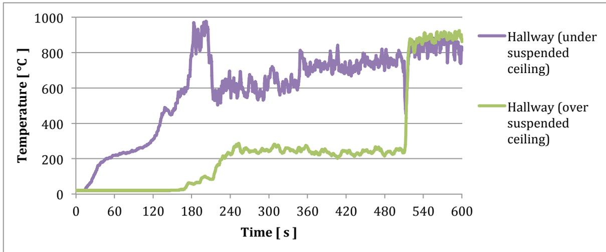
Figure 7-2 Temperature – time curve. Over and under suspended ceiling in hallway. Window: 1.2m x 1.6m
