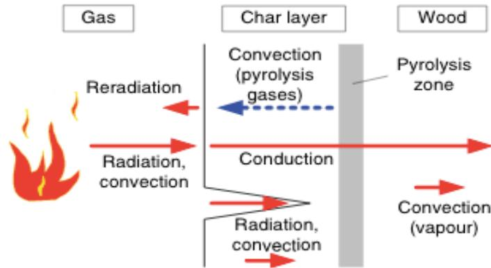
**Figure 4-7 Heat flux components in fire-exposed semi-infinite wood slab due to external heat source (König, 2006)**
