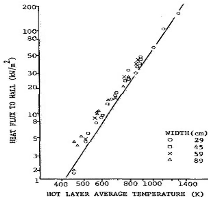
Figure 4-18 Correlation between the average temperature of the hot layer of gases in a compartment and the heat flux on the walls of the compartment (Tanaka et al., 1986)
