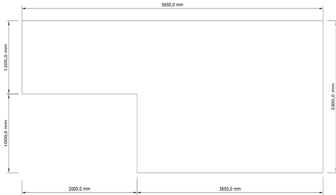
**Figure 6-2 Sketch presenting the measurements of the floor area used in calculations. The measures have been carried out manually and may deviate some from the floor plan**
