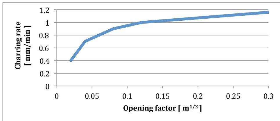
Figure 4-20 Effect of opening factor on the charring rate
