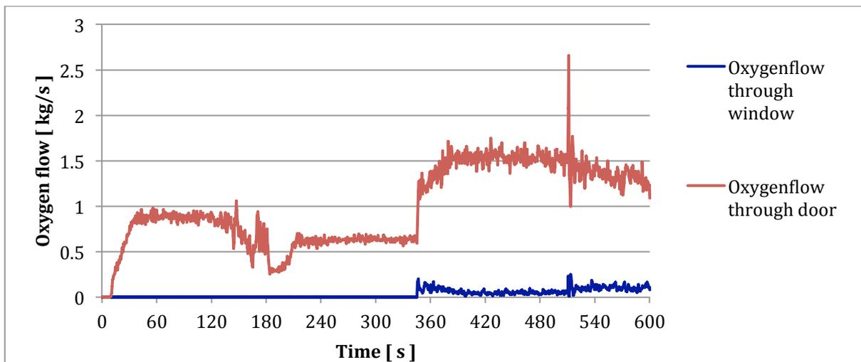
Figure 7-3 Oxygen flow through window/door during the first ten minutes of the simulated fire. Window: 1.2m x 1.6m
