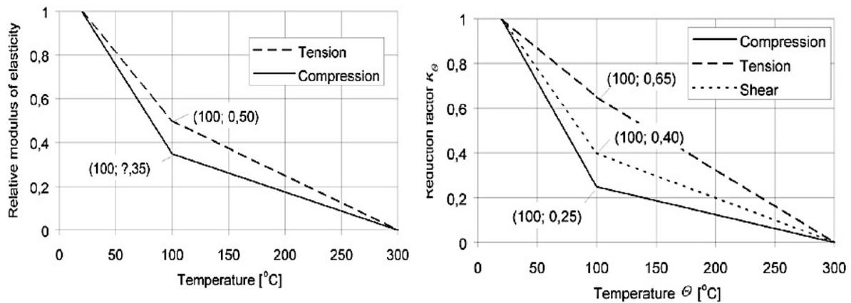
**Figure 3-11** The effect of temperature on modulus of elasticity and the reduction factor for strength parallel to the grain of softwood (Norsk Standard, 2010)
