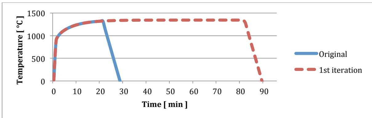
**Figure 4-5 Iteration of parametric temperature-time curve**
