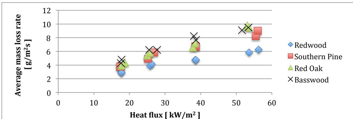
**Figure 4-11 Average mass loss rate for various heat fluxes (Tran and White, 1992)**
