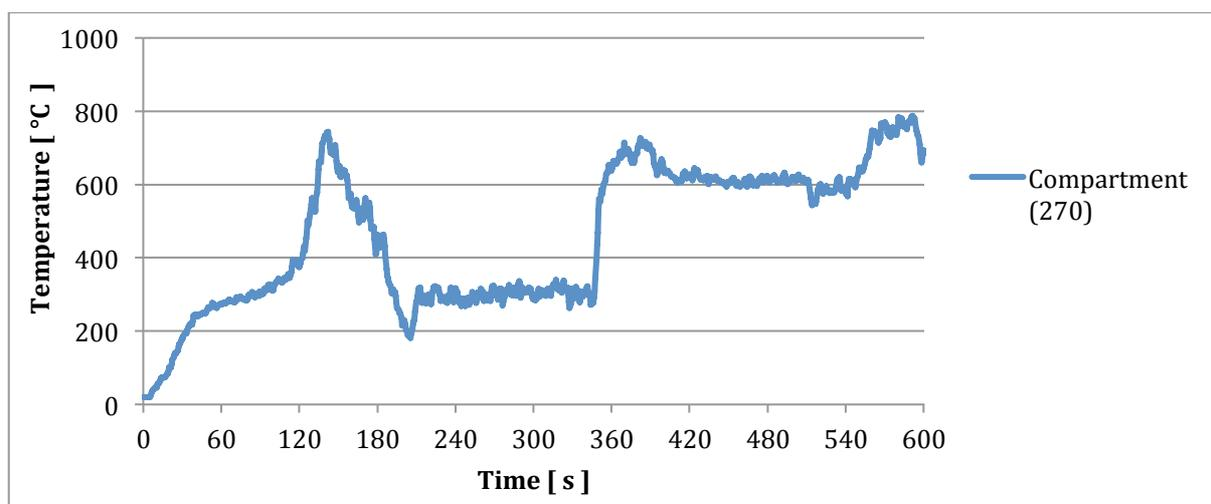
Figure 7-1 Temperature – time curve. 270 cm above the floor in the compartment. Window: 1.2m x 1.6m
