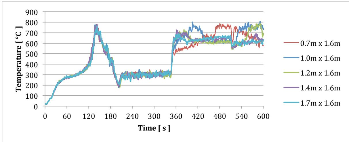
**Figure 7-5 Temperature – time curves for the first ten minutes of the fire simulated in the compartment modelled.**
