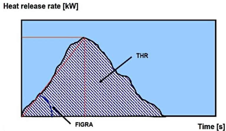
Figure 3-1 Heat release rate and FIGRA index. Used to classify a materials reaction to fire.
