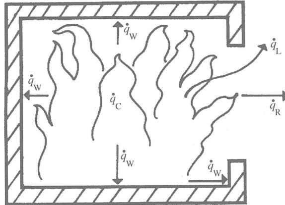
**Figure 3-7 Illustration of heat losses during a fully developed compartment fire (Drysdale, 2011; Petterson et al., 1976)**
