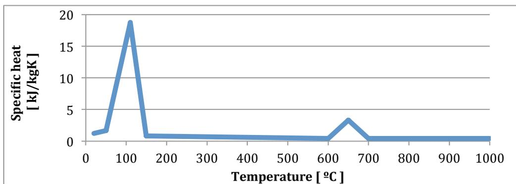
Figure 3-16 Specific heat of gypsum plaster, for varying temperatures
