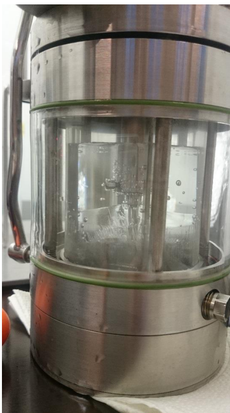
Figure 7.7-2 Picture of frozen reaction mass (H 2 O) after a unsuccessful scanning experiment
