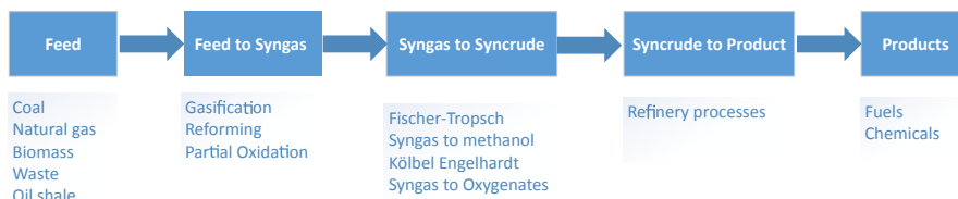
Figure 2.1: Simple block diagram of a Gas to Liquid process [33]
