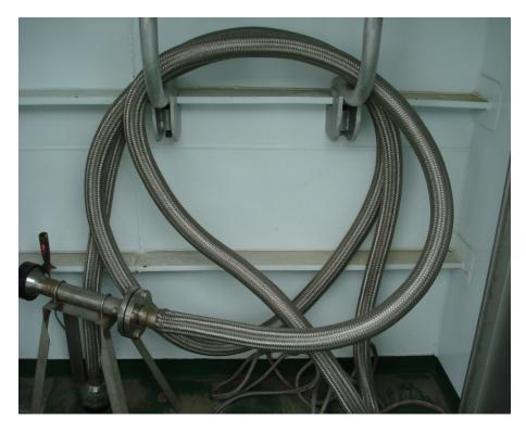
Figure 74: Bunkering Line on MF Korsfjord
