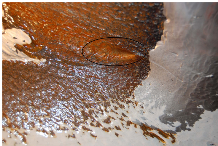
(b) Typical ring-grooves near the stay vane leading edge
