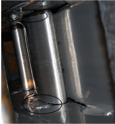
Figure 4.3: Horse shoe vortex of facing plates in the guide vane channel, Cahua power plant
