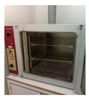
Fig. 4.9: Oven used to determine the moisture content of the samples
