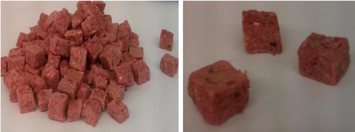
Fig 6.14: Standard samples 20 mm dried at 25°C
