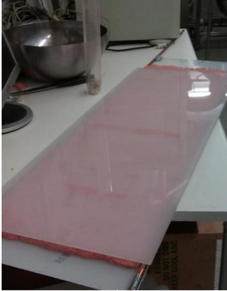
Fig. 4.2: Material layer distributed over a methacrylate sheet before freezing
