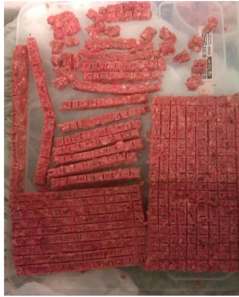
Fig. 4.3: Detail on cutting of the frozen layer into 10mm long slab shaped particles
